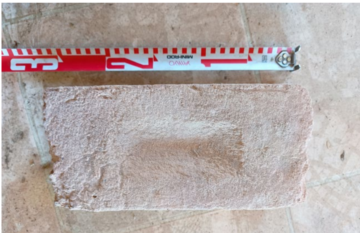
Plate 48. Size and form of the sandstock bricks, including shallow, irregular frog, poor facing andarris edge. A probable partial thumb print in the handmade fabric is seen at lower right (Source: Archive Heritage)
