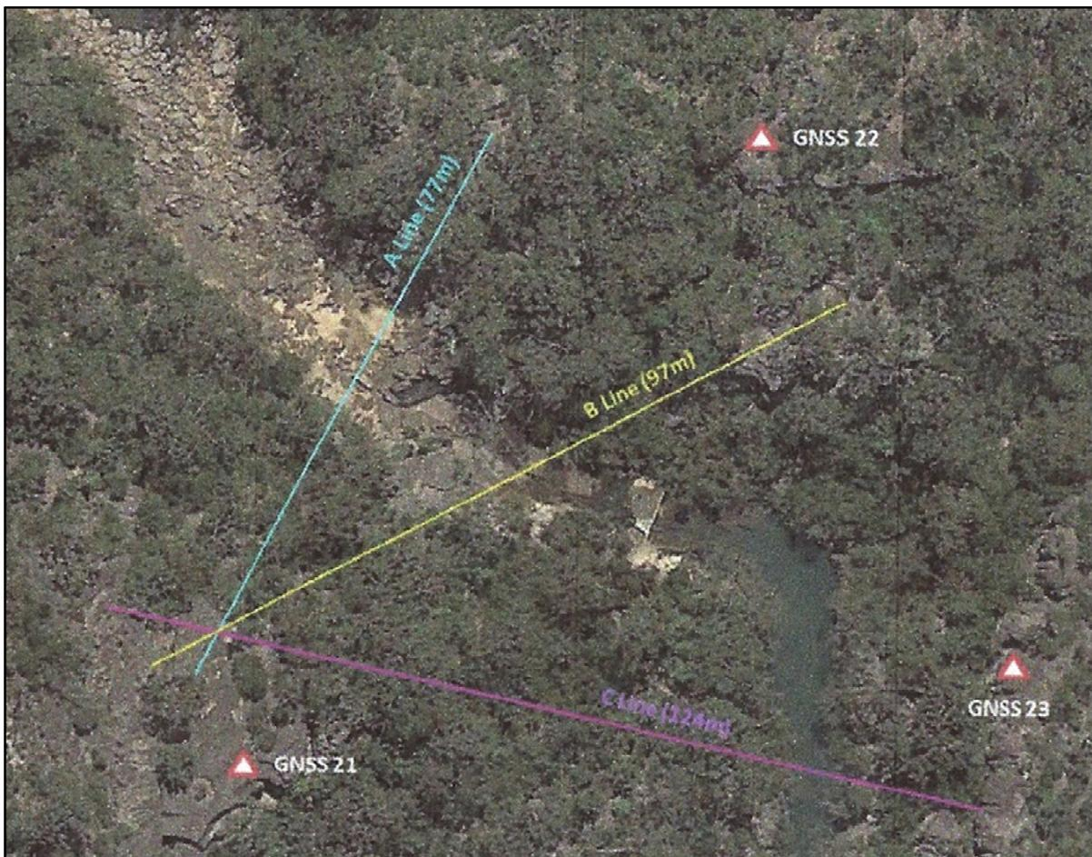
**Figure 4.14 High precision survey lines across Eastern Tributary**
