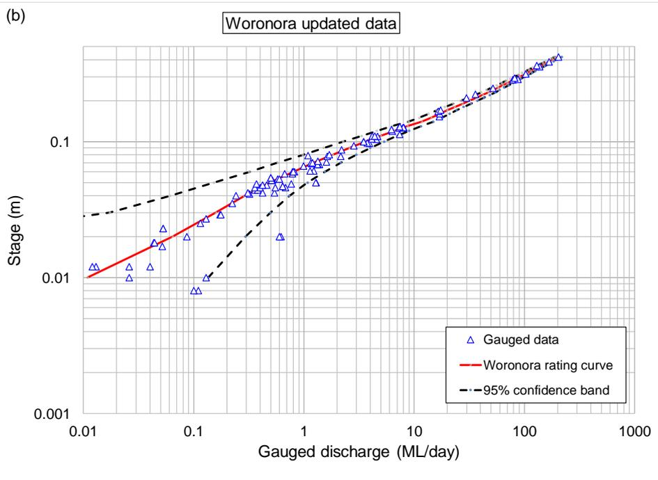
**Figure A2. Rating curve for (a) Waratah Rivulet (GS2132102) and (b) Woronora River (GS2132101) showing the 95% uncertainty band**
