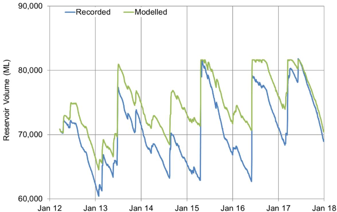
**Figure 9 Simulated Reservoir Volume with Systematic Rainfall Error**
