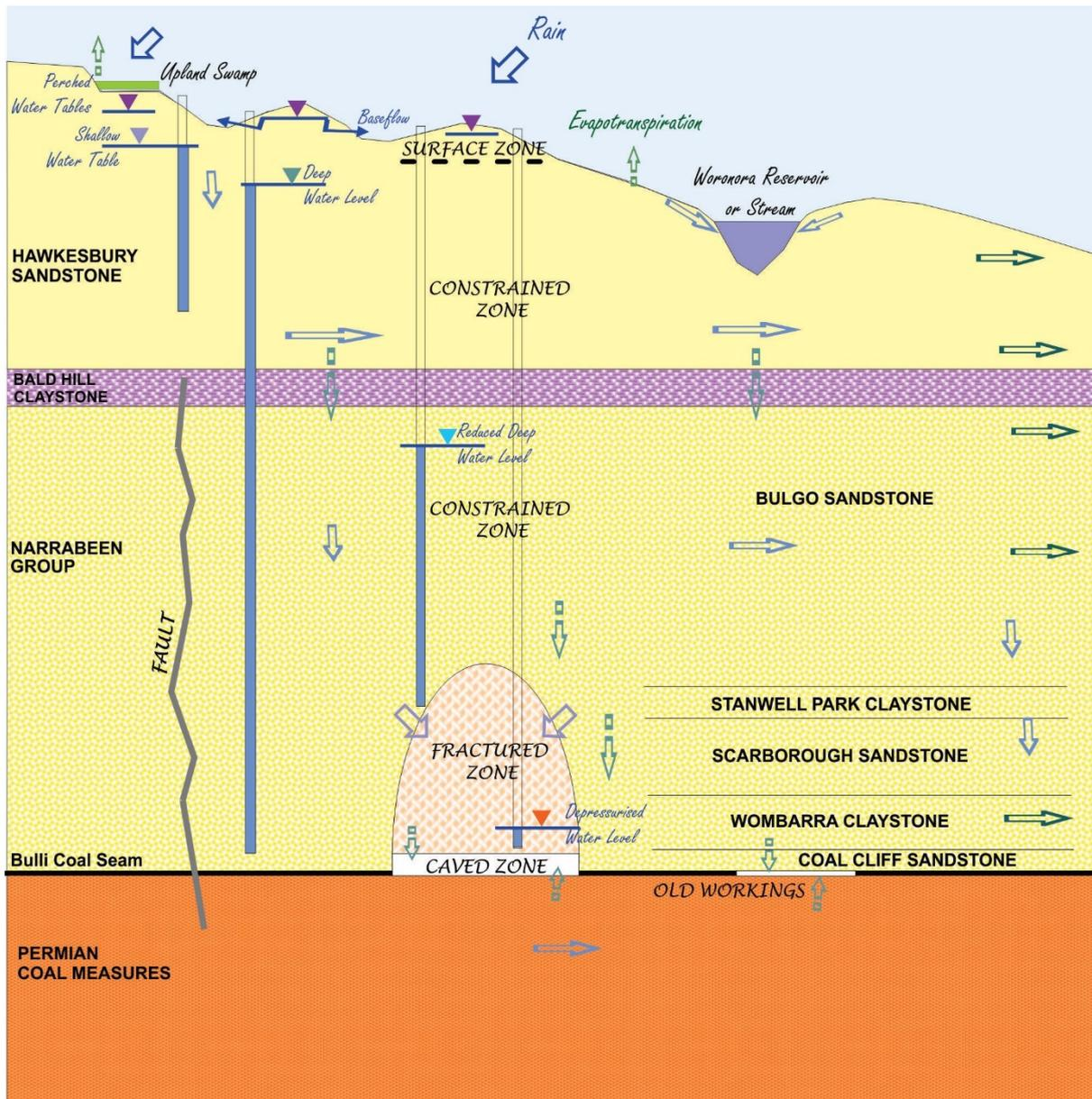
**Figure 2.1. Conceptual groundwater system for Metropolitan Coal mining conditions**
