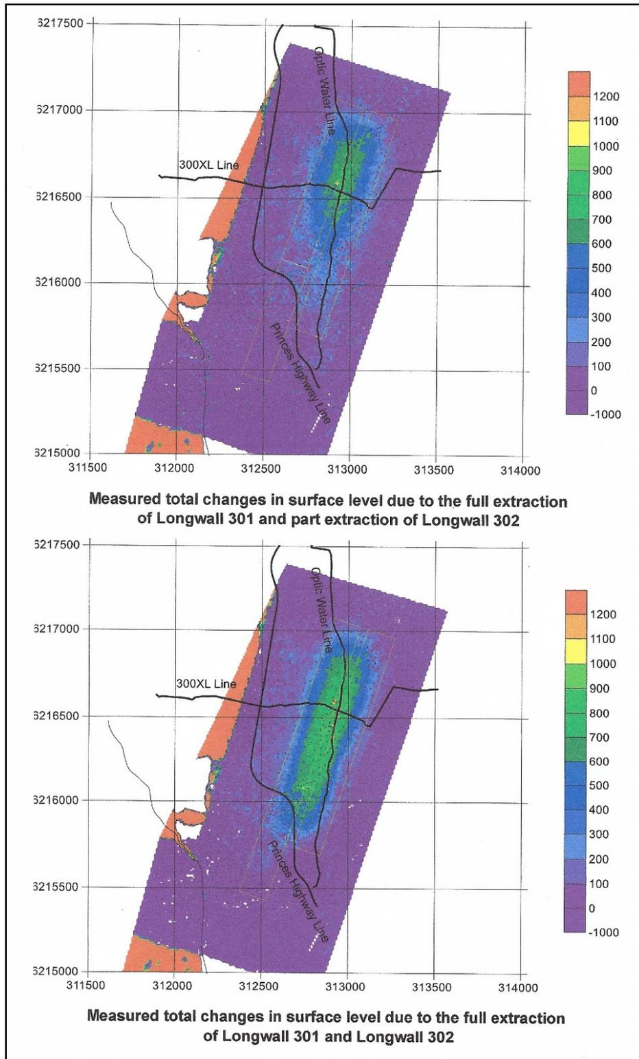
**Figure 4.12 LIDAR survey results after LW301 and LW302**
