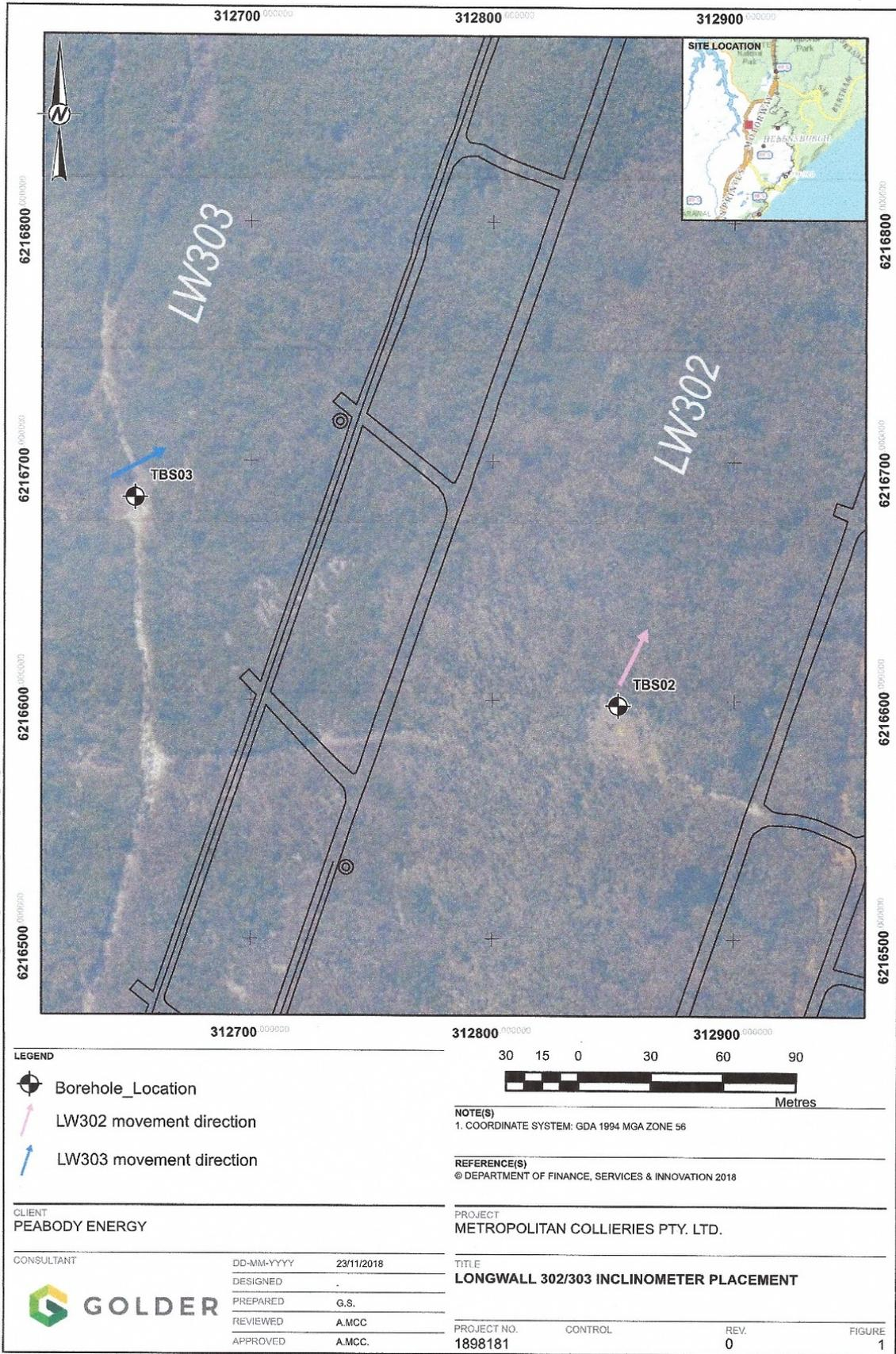
**Figure 4.2 Location of borehole inclinometers TBS02 and TBS03**
