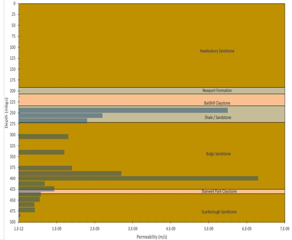
**Figure 4.6 LW302 overburden conductivity test results – pre- and post-mining**
