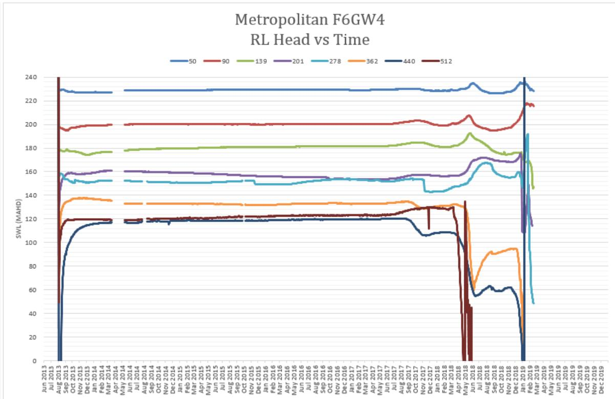
**Figure 5.6 Piezometer levels over the period 2013 to early 2019 at borehole F6GW4**
