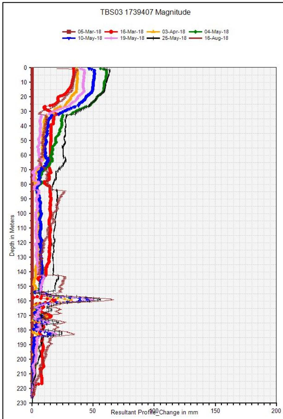
**Figure 4.5 Borehole Inclinerometer TBS03 results**
