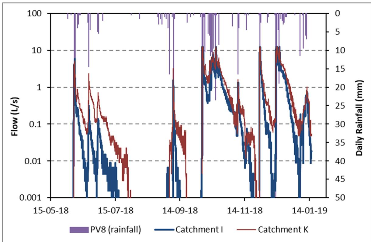
**Figure 6.5 Measured hydrographs at flow monitoring stations I and K and observed rainfall at station PV8**
