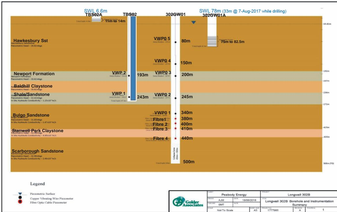
Figure 5.2 Longwall 302 borehole and Instrumentation
