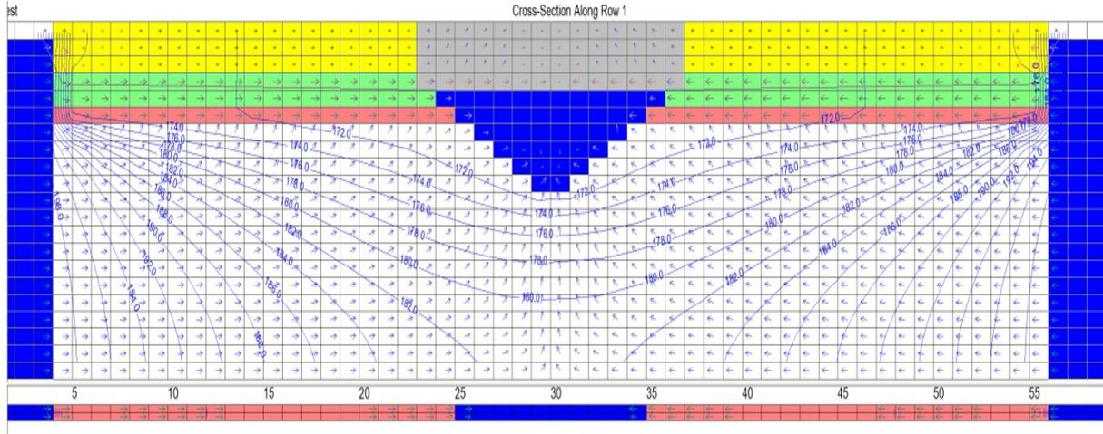
**Figure E1. 2D 10 m thick idealised layered section with variable saturation MODFLOW numerical model with variable hydraulic conductivity with depth and Woronora Reservoir indicating flow vectors and hydraulic head contours.**
