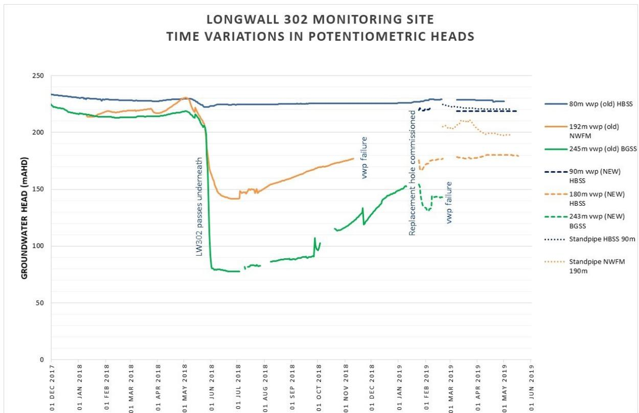
**Figure 5.4 Extended piezometer pressure heads recovery in older 2018 and newer VWP's in 2019**
