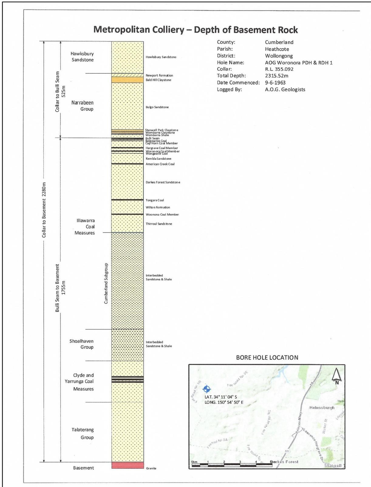
**Figure 4.7 Surface to basement geological section – Metropolitan Coal**
