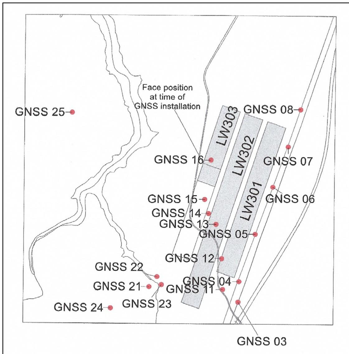
**Figure 4.13** GNSS survey station array installed around LWs 301 – 303
