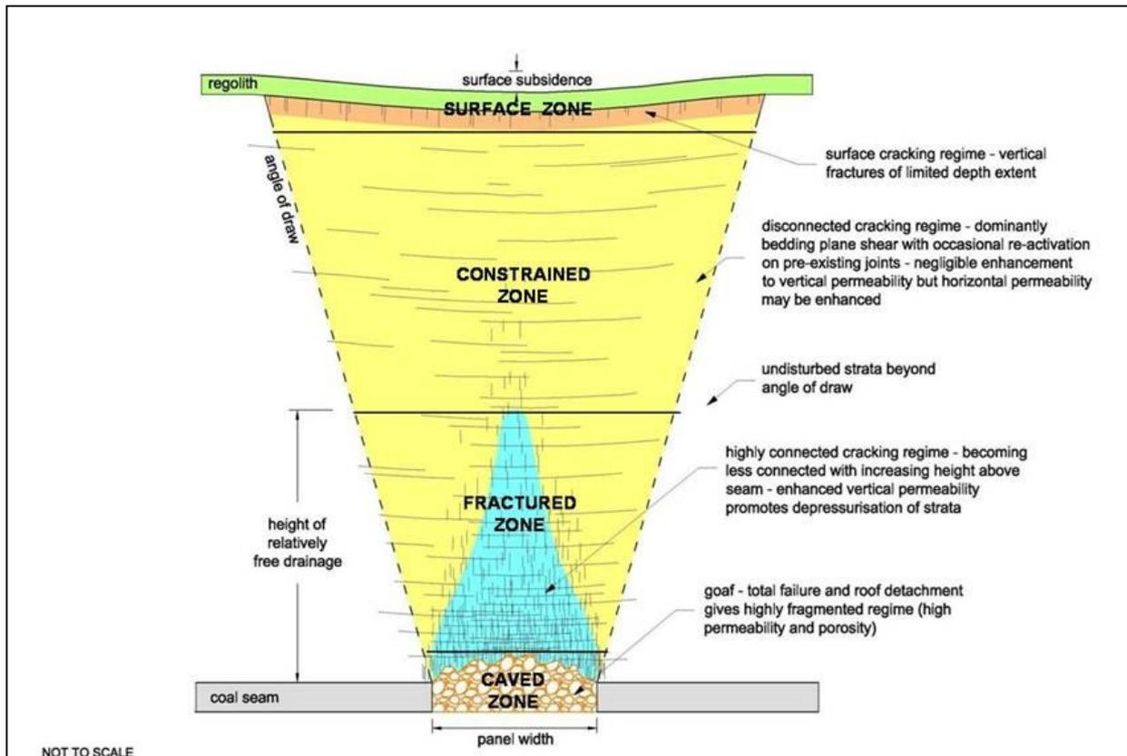
**Figure 4.1 “Height of Fracturing” concept.<sup>7</sup>**
