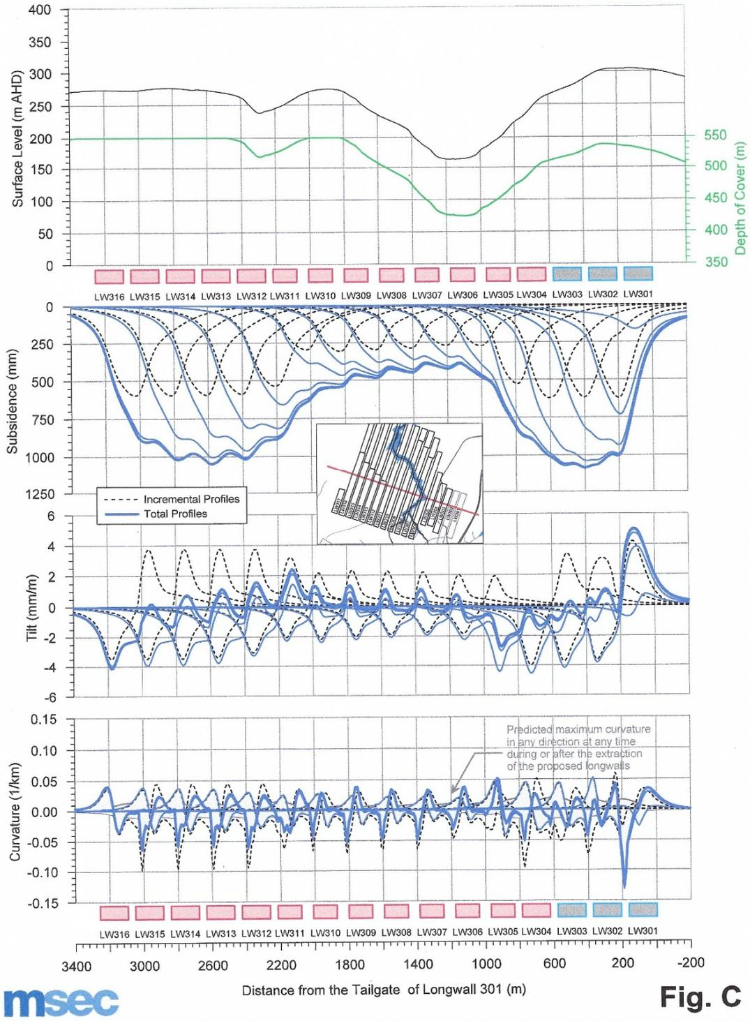
**Figure 4.11** Predicted subsidence along a centreline cross-section – LWs 301 to 317
