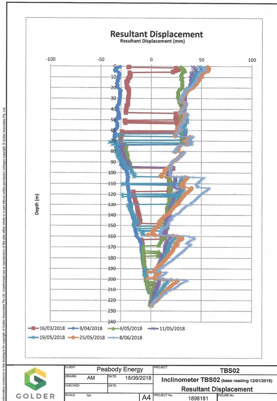
**Figure 4.3 Borehole inclinometer TBS02 results**
