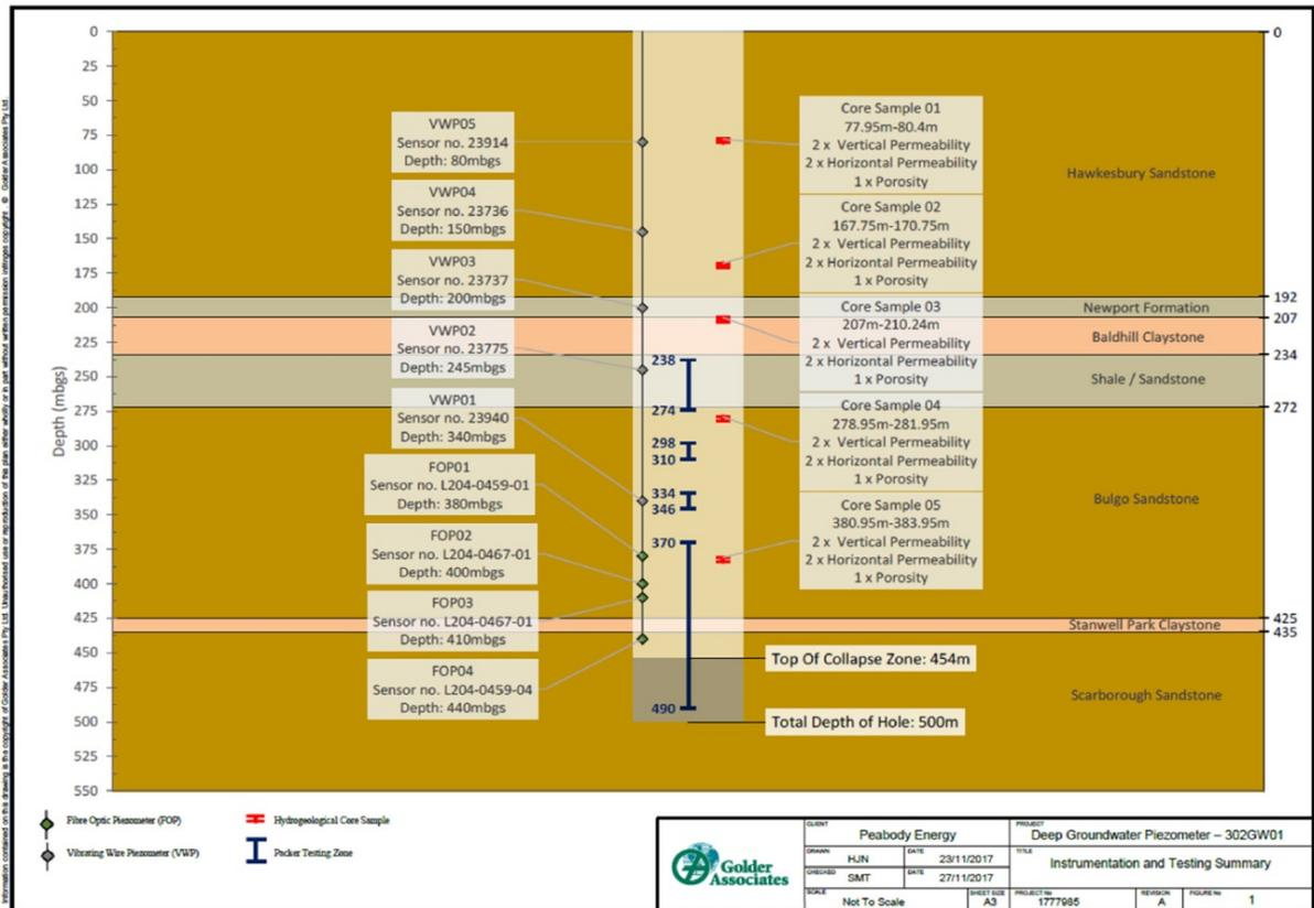
**Figure 5.7 Packer tests and Hydraulic conductivities of Core Samples**
