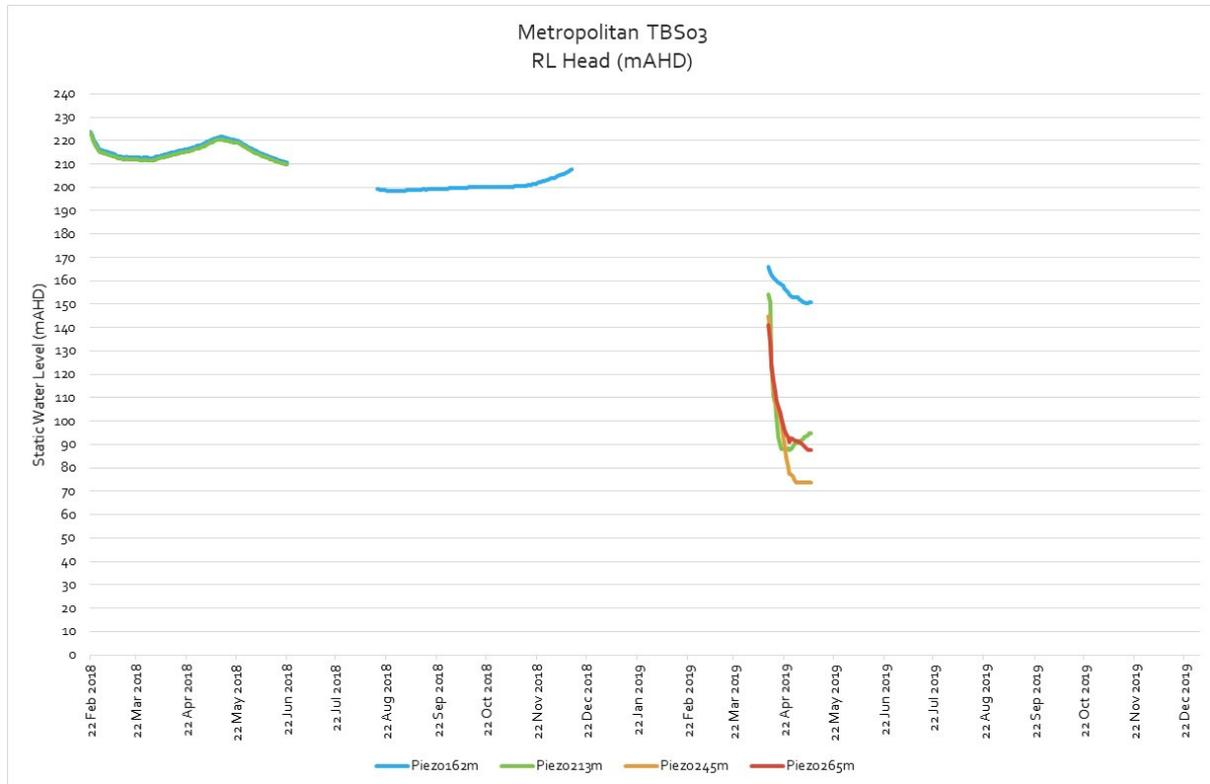
**Figure 5.5 TBSO3 piezometer static water levels**
