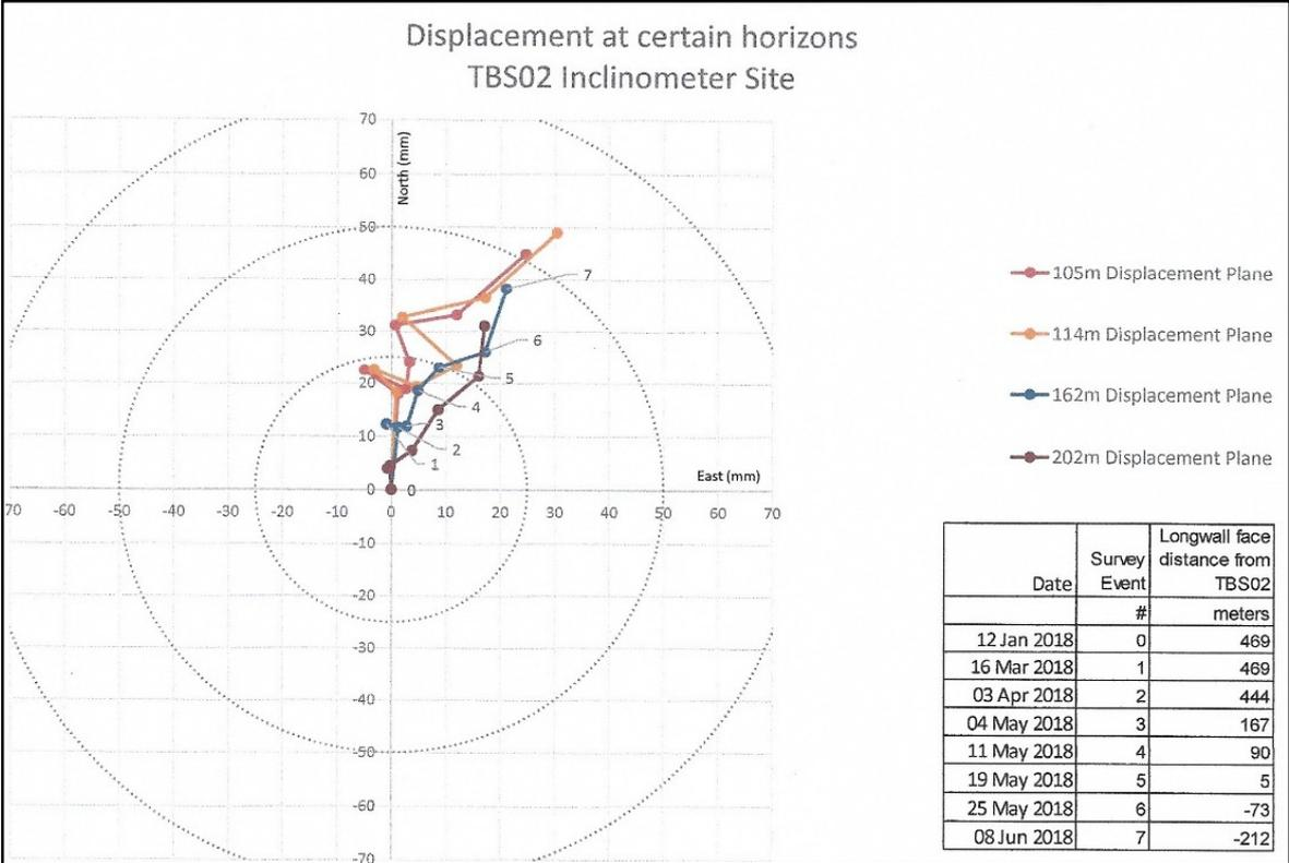
**Figure 4.4 Inclinometer TBS02 – direction of movement for selected bedding plane horizons**
