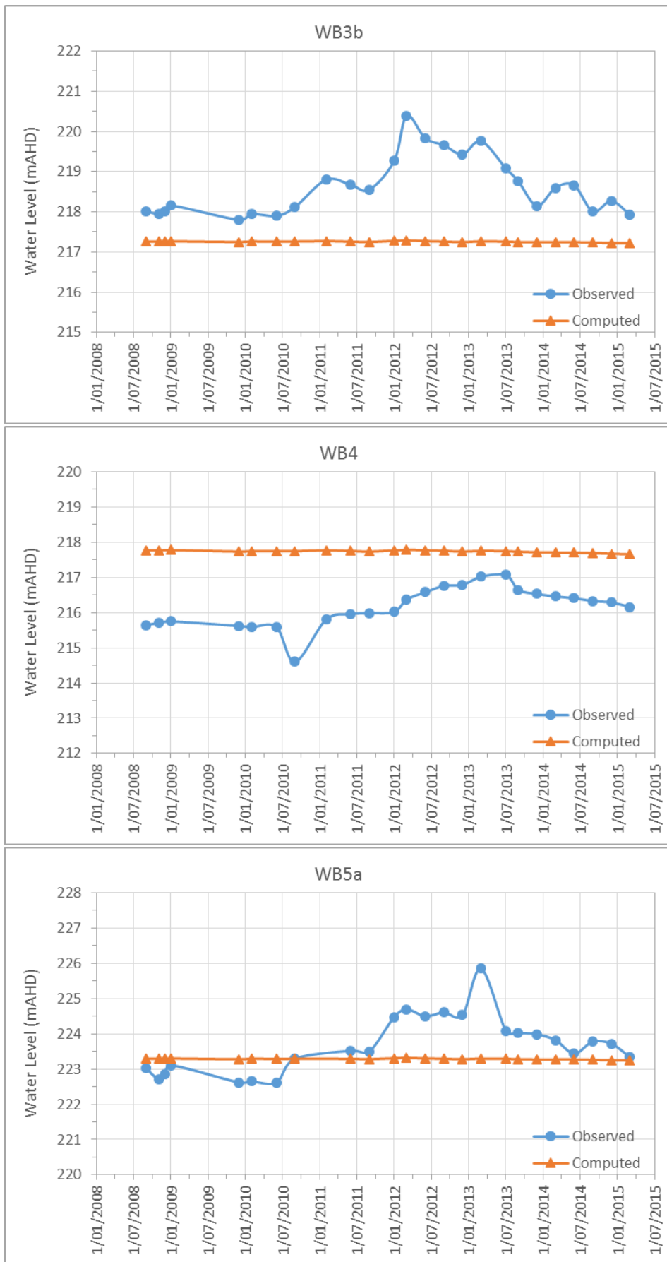
Figure K10. Observed and Simulated Hydrographs - Version 4 Model – Group 2: WB3b, WB4, WB5a
