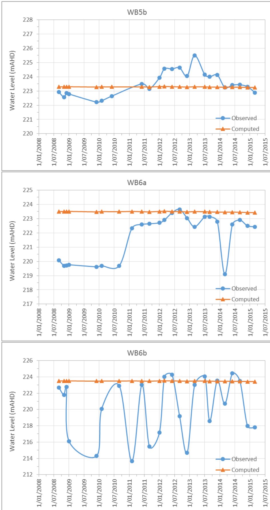
Figure K11. Observed and Simulated Hydrographs - Version 4 Model – Group 2: WB5b, WB6a, WB6b
