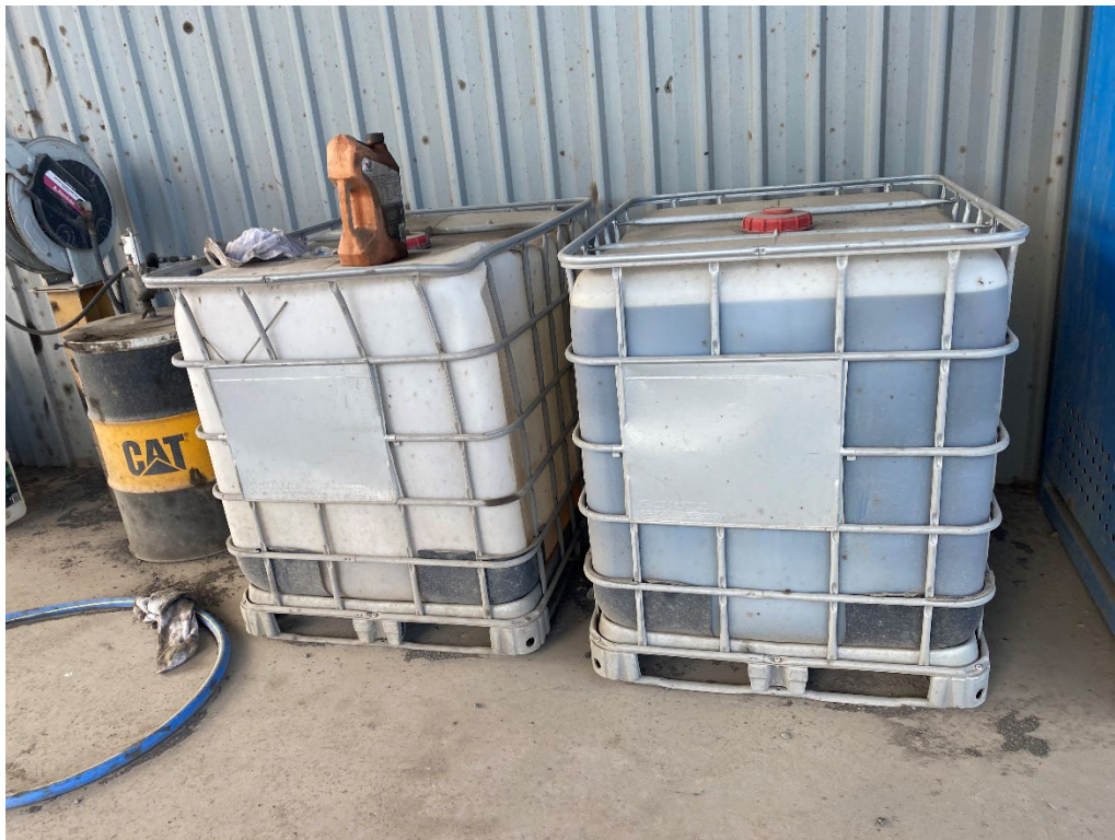
Photo 8: Full hydrocarbons not stored correctly in workshop
