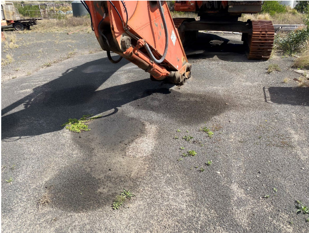
Photo 7 : Visible hydrocarbon leaks under old machinery in “Graveyard”
