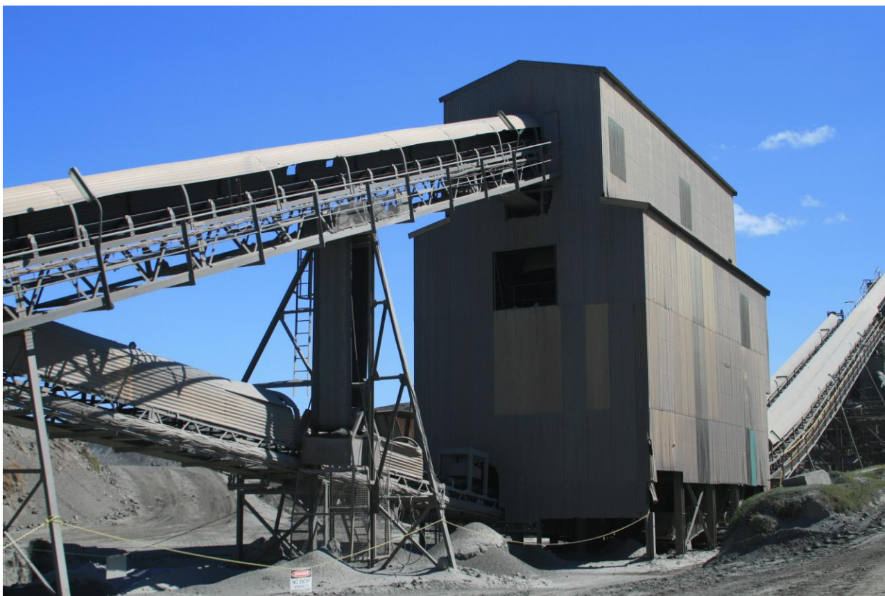
Existing crushing and sorting plant with conveyors
