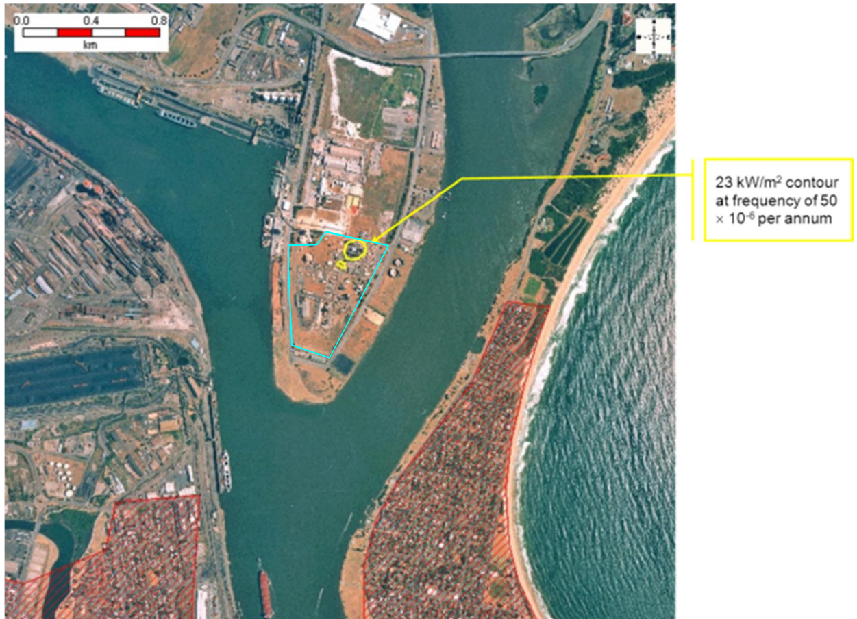
Figure VIII-7: Thermal Radiation - Property Damage Risk
