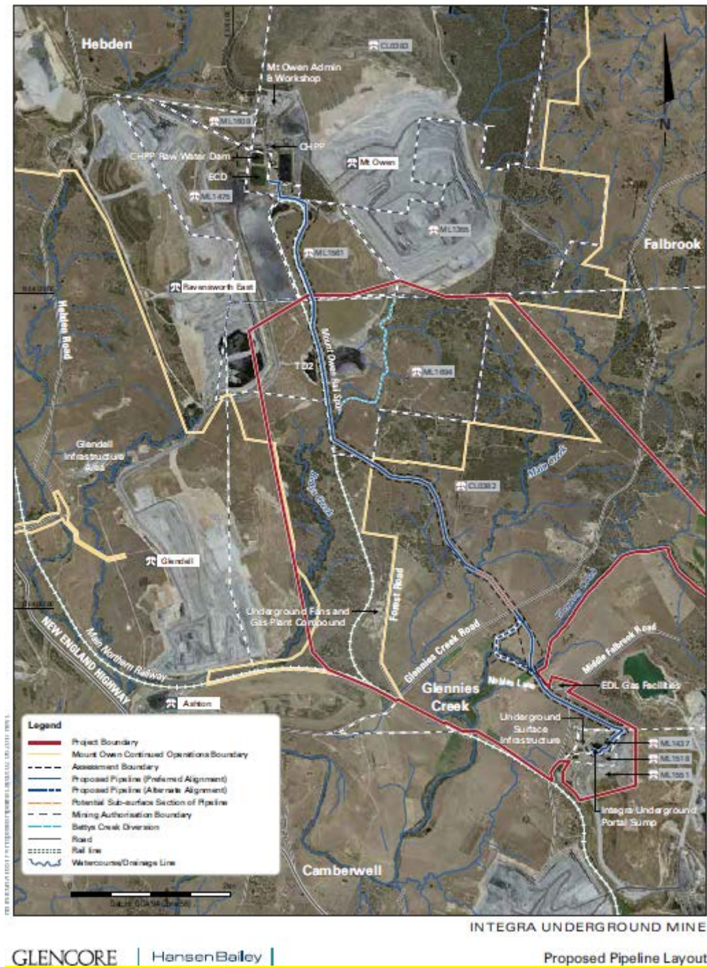
Figure 3: Water Pipeline Infrastructure
