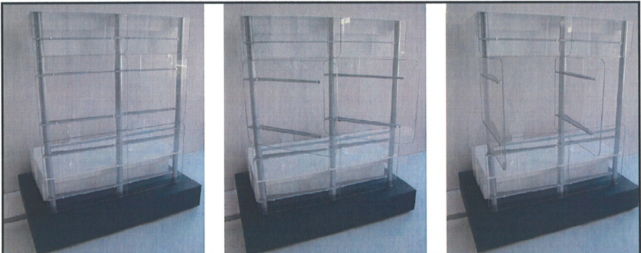
Figure 4: Model of glass panels in closed and open forms
