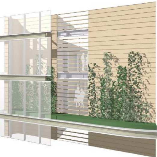
core facade showing glazed lift lobby, and planting to core
