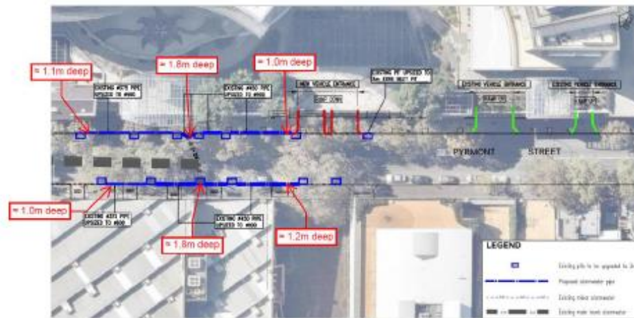
Figure 1 - Proposed Stormwater Works on Pymont Street
