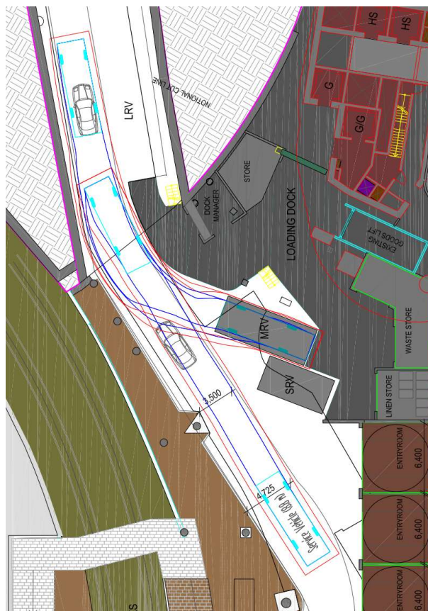
Figure 3.11: Proposed Star Events Loading Dock Upgrades
