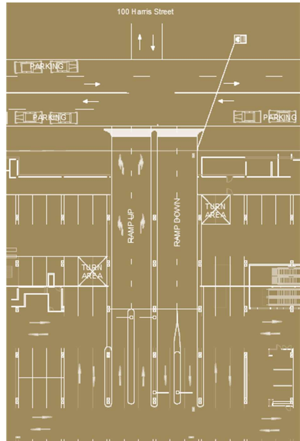
Figure 3.2: Pymont Street Entry Ramp layout
