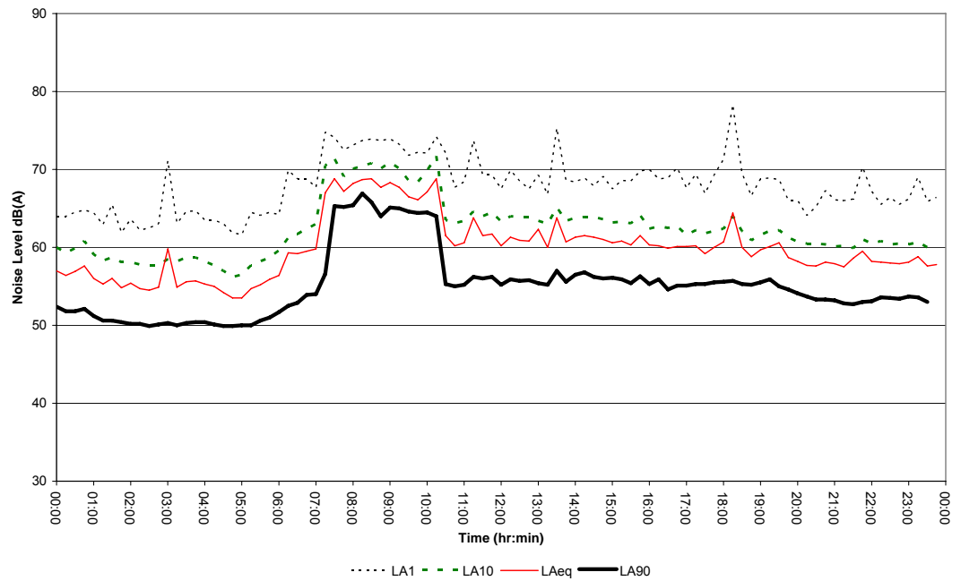
Figure 8: Average Weekday Noise Levels, 29 May 2008 to 18 June 2008, Switching Station Site, dB re 20 \mu Pa
