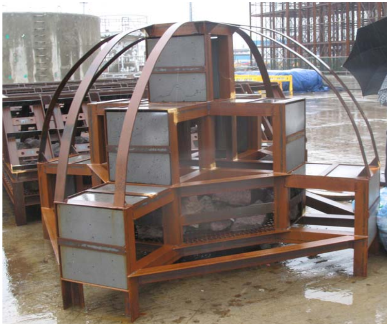
Figure 2: Examples of ‘design specific’ artificial reef units used in South Korea - (a) individual concrete cube units have been used extensively; (b) using steel means greater complexity in artificial reef unit design can be achieved (images: NSW DPI).
