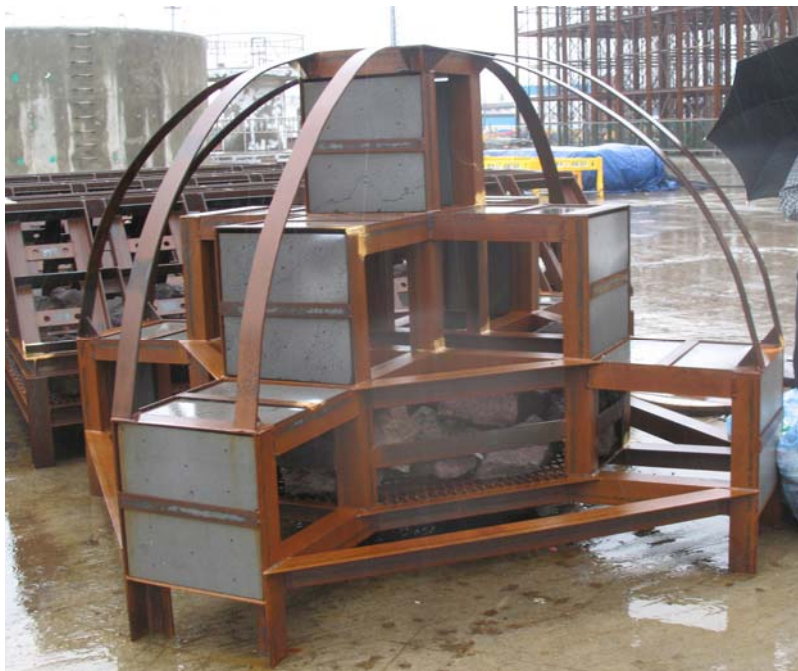
Figure 2: Examples of ‘design specific’ artificial reef units used in South Korea - (a) individual concrete cube units have been used extensively; (b) using steel means greater complexity in artificial reef unit design can be achieved (images: NSW DPI).
