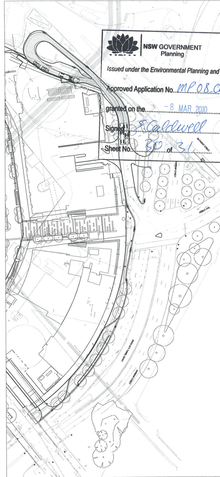
USER DEFINED 14m SEMI TRAILER @ 15Kmh/h BASED ON AUSTRADS 15.0m SEMI TRAILER VEHICLE TEMPLATE (TRAILER LENGTH REDUCED)
