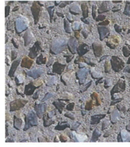
EXPOSED AGGREGATE CONCRETE Portland grey cement with high quality 7-14mm aggregate. Aggregate to be custom mix of crushed stones including quartz, basalt and porphyry
