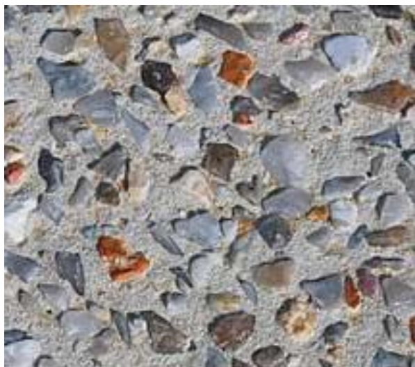
EXPOSED AGGREGATE CONCRETE Portland grey cement with high quality 7-14mm aggregate. Aggregate to be custom mix of crushed stones including quartz, basalt and porphyry
