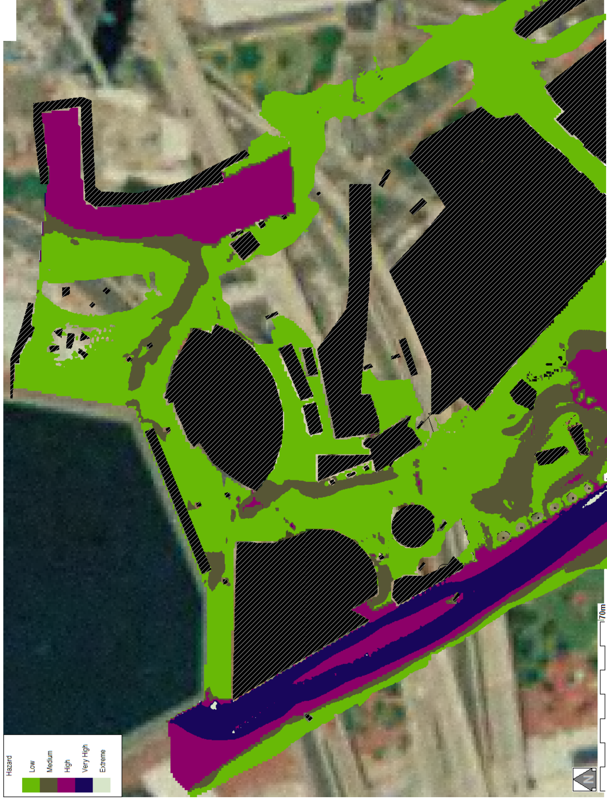
FLOOD STUDY ADDENUM 3 DARLING HARBOUR FLOOD HAZARD PROPOSED 100 YEAR ARI 60 MIN STORM
