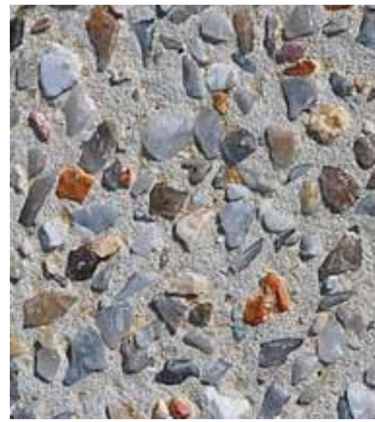
EXPOSED AGGREGATE CONCRETE Portland grey cement with high quality 7-14mm aggregate. Aggregate to be custom mix of crushed stones including quartz, basalt and porphyry
