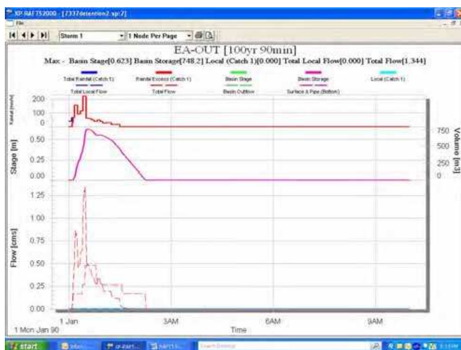
Figure 7 – EA Site 100yr ARI Post Development (With Detention) Hydrograph
