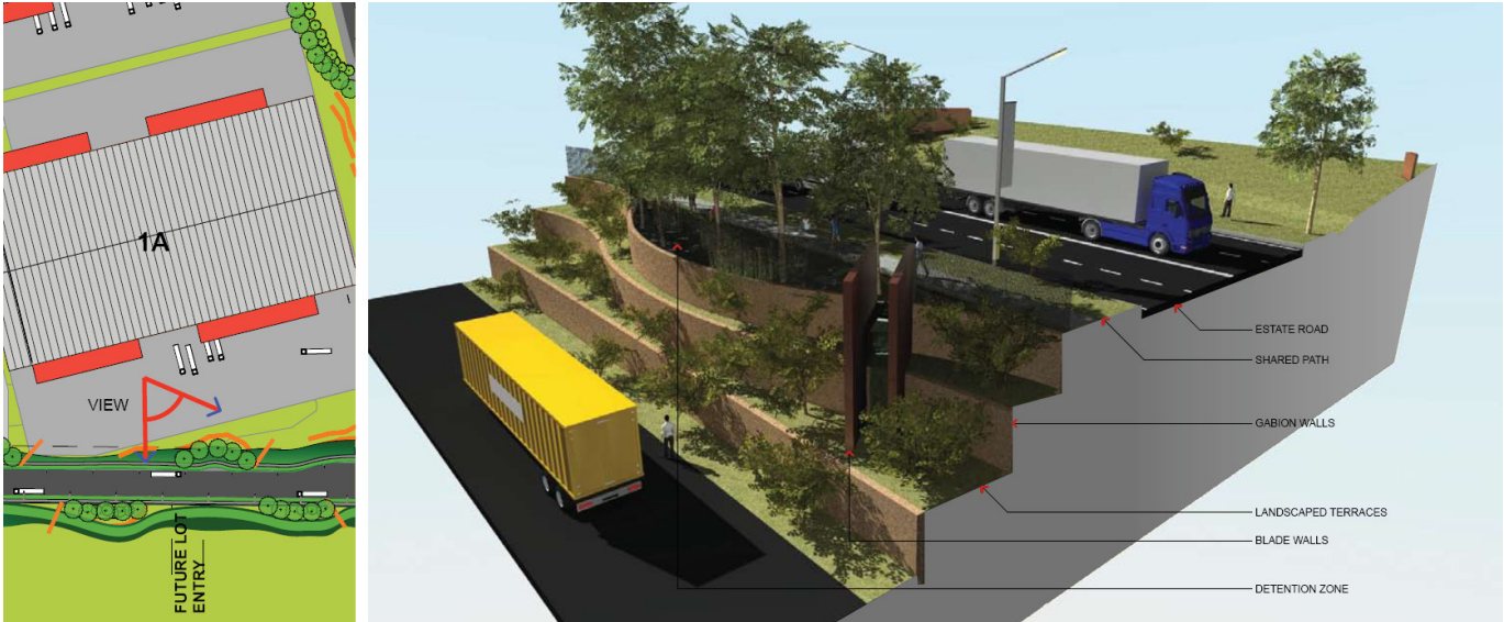
Figure 12: DHL Landscape Plan – Detailed Section of Retaining Wall adjacent Old Wallgrove Road
