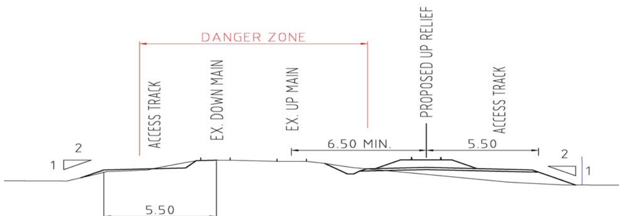
Figure 3-4 Type 1 Cross Section – Extended Formation (At Grade)
