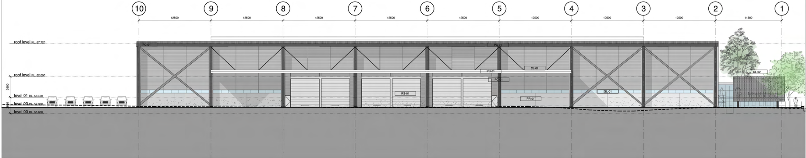
02 West Elevation Warehouse & Warehouse Office 1:200
