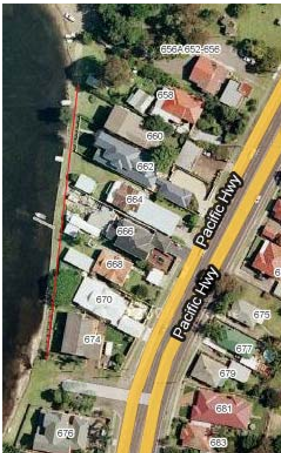
Plate 3 Red line denotes the waterline in earlier periods. The straight retaining wall retains the sewer line and fill.
