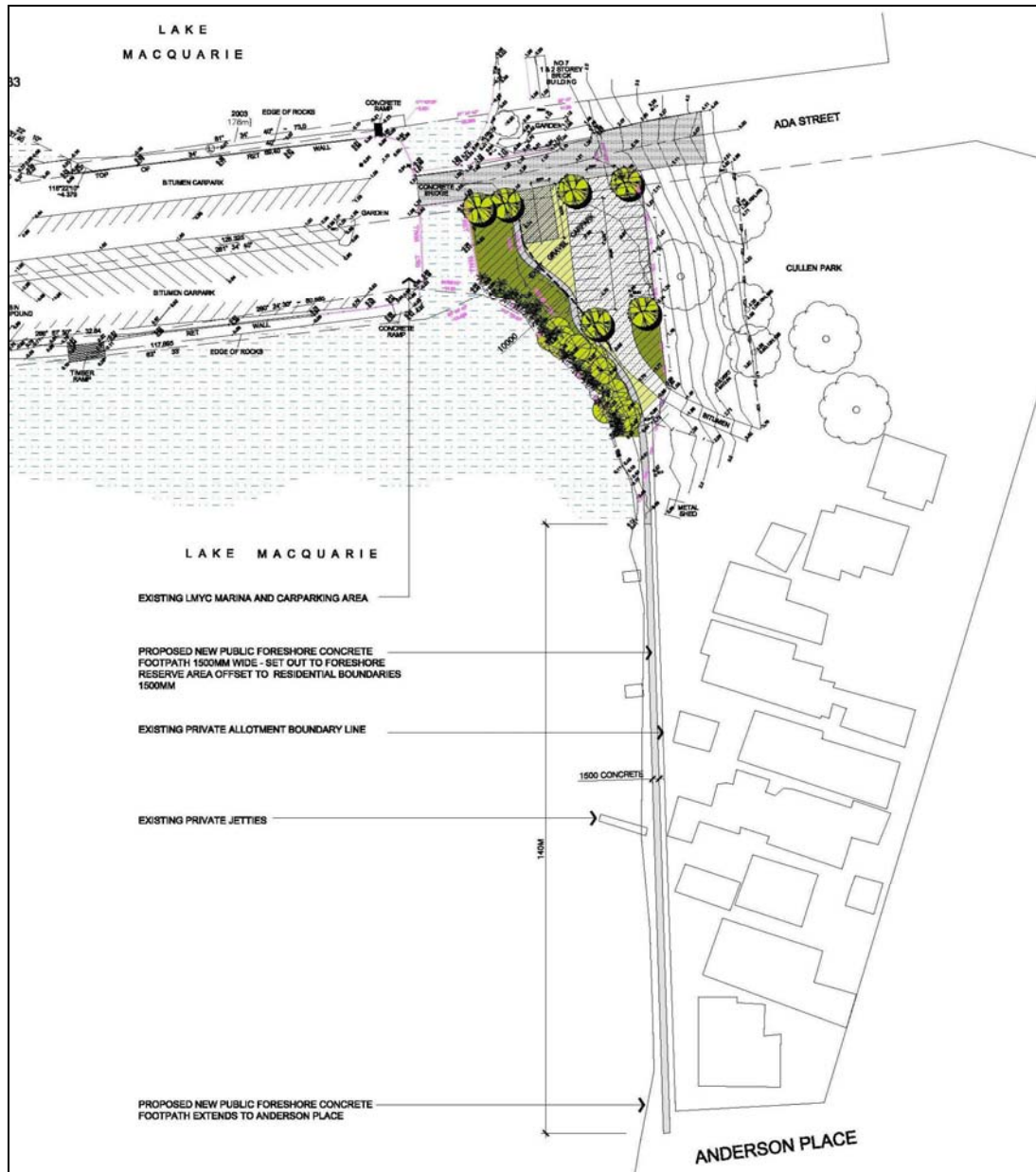
Figure 9 The proposed cycle / pedestrian path connecting the Yacht Club to Anderson Place. The path lies over a sewer main.
