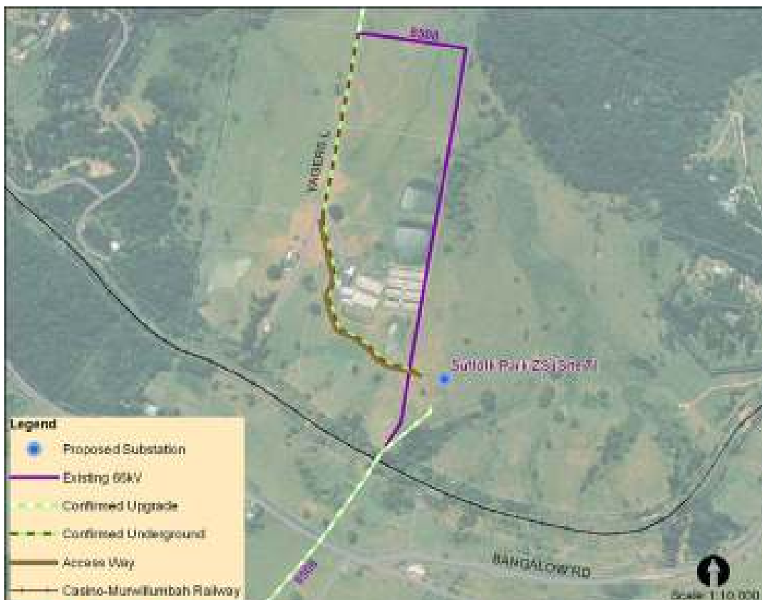
Figure 3: Proposed Alignment at Suffolk Park Substation
