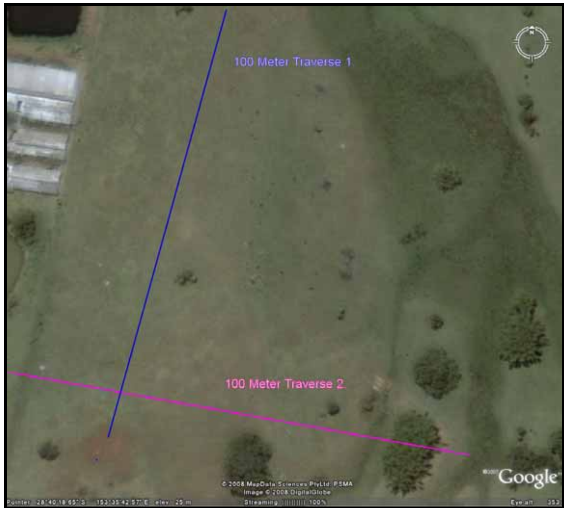
Suffolk Park Site 7. Soil Resistivity Traverses.
