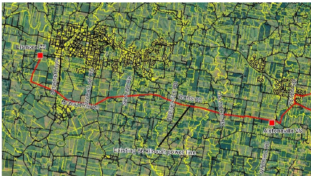
Aerial view of proposed 132kV powerline route
