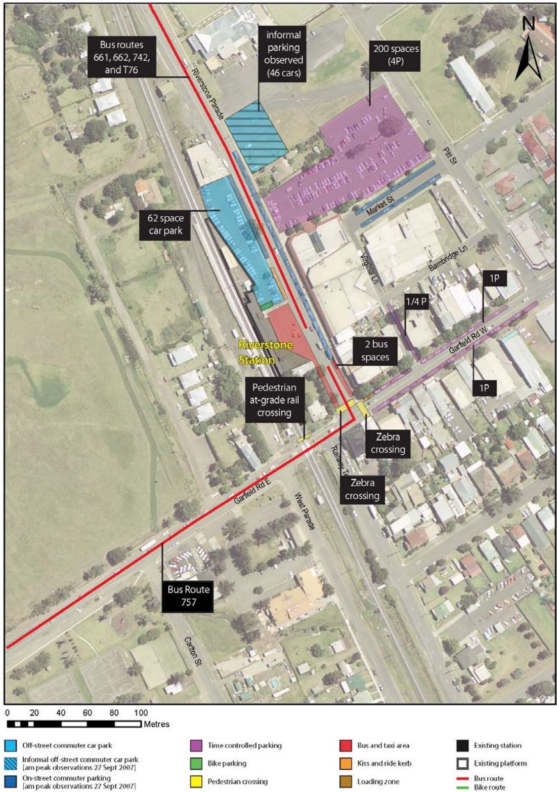
Figure 2-10 Existing transport facilities at Riverstone Station
