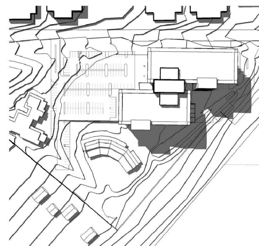
3 21st MARCH - 3PM AZIMUTH ANGLE = 61° WEST OF NORTH ALTITUDE ANGLE = 36° ABOVE THE HORIZONTAL
