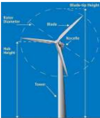
Figure 2: Impression of typical wind turbine (82m rotor installed on an 80m tower)
