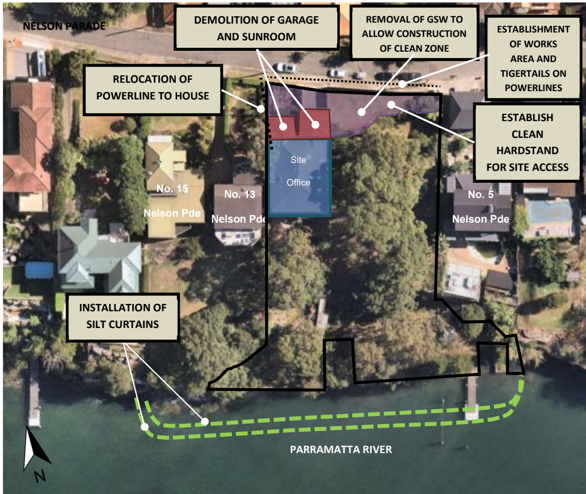
Figure 1: Site Establishment Works
