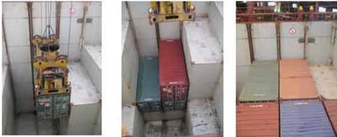
Figure 2: Placement of containers in under deck holds (Photo courtesy of the Guide for Safe Transport of UOC )
