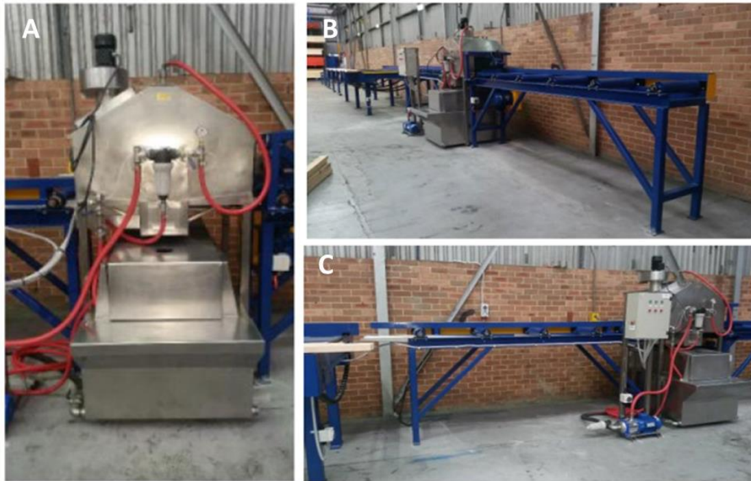
Figure 2 | Proposed H2F Timber Spray System Model, including A: Linear Sprayer including an enclosed booth, B: Infeed Roller Conveyor & C: Outfeed Roller Conveyor
