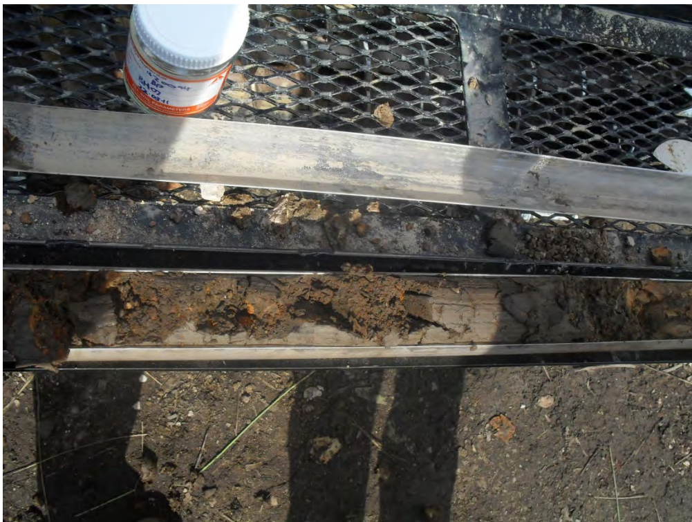
Photo 4 Soil material observed from the soil core at BH07.
