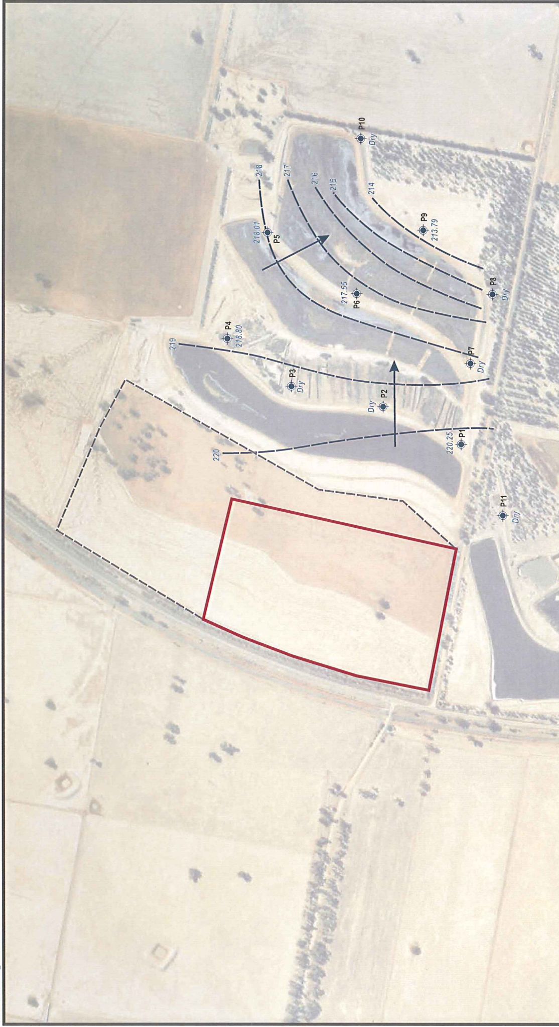
Figure 5 Groundwater Standing Water Levels: Deep Aquifer Summer 05/01/2006
