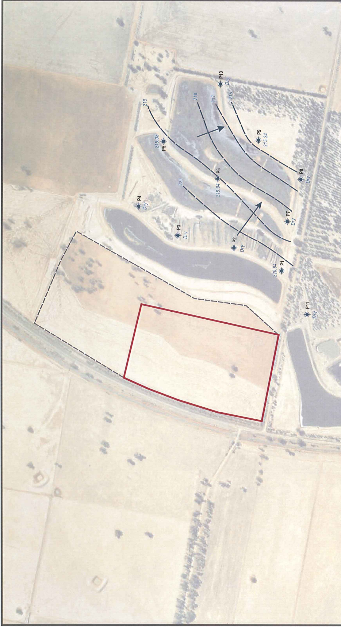
Figure 3 Groundwater Standing Water Levels: Deep Aquifer Summer 07/01/2004 Riverina Oils and Bio Energy Pty Ltd Groundwater Review Integrated Oilseed Processing and Biodiesel Plant
