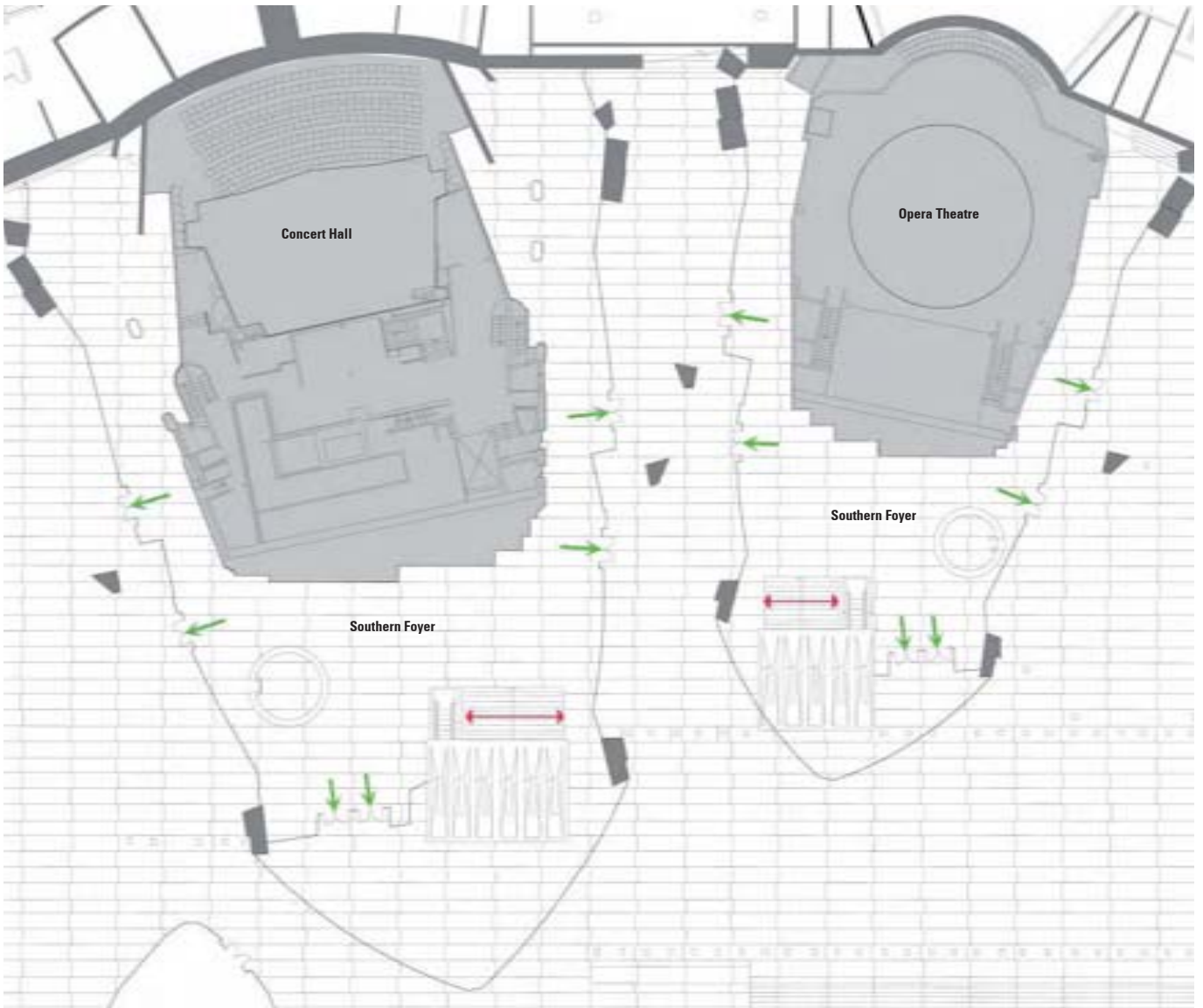
Level 42 Southern Foyer fire egress exits
