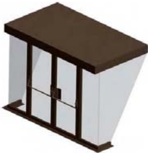
Isometric view of typical existing door niche
