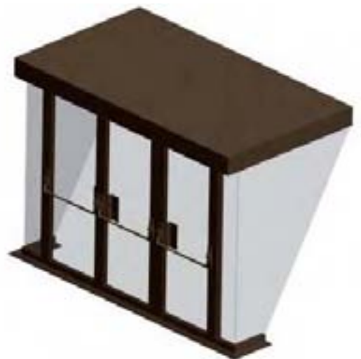
Isometric view of typical proposed door niche
