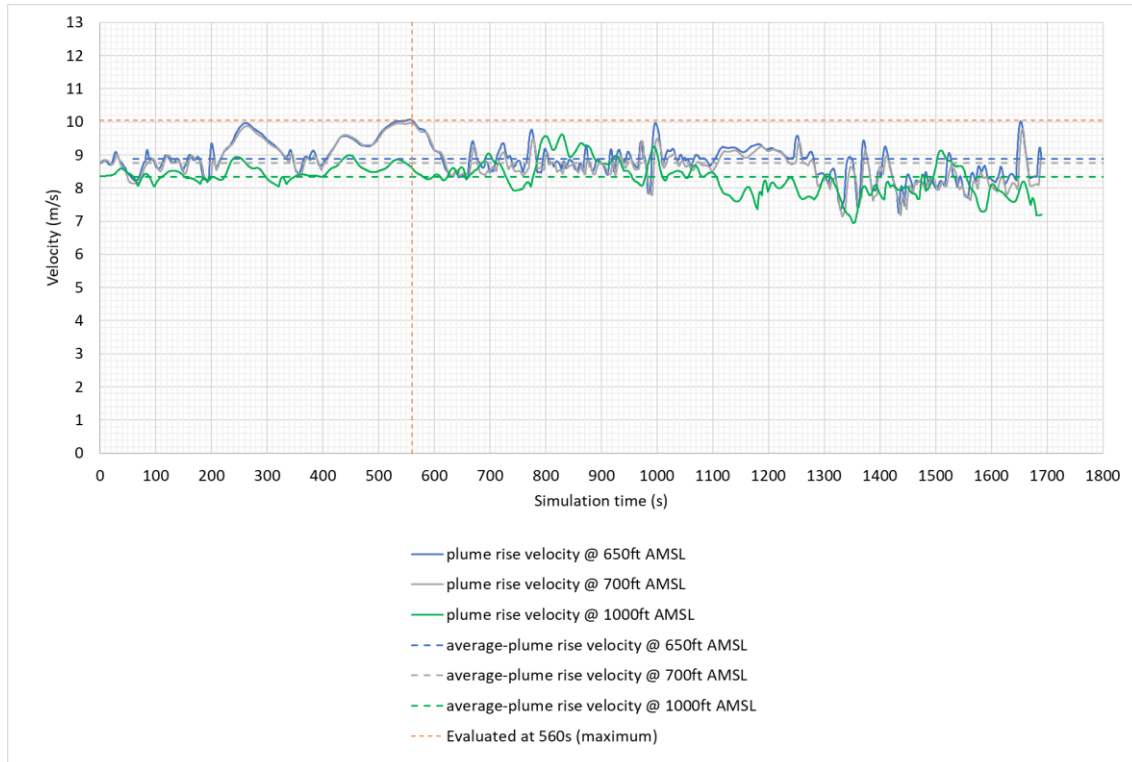
Figure 9. Monitored peak velocities at different heights depending on the simulation time – Calm wind case. The dashed orange vertical line illustrates the simulation time chosen for the detailed analysis.
