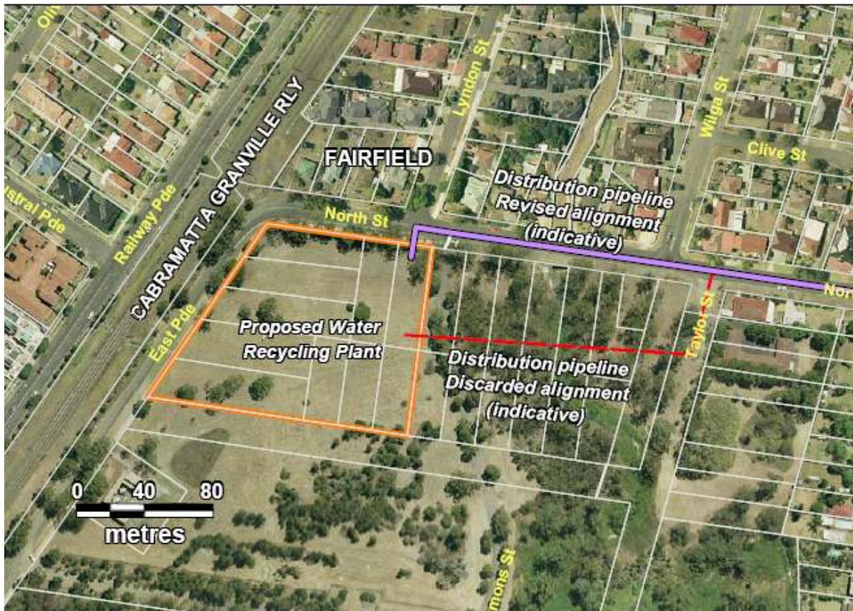
Figure 6: Revised distribution pipeline alignment on North Street, Fairfield
