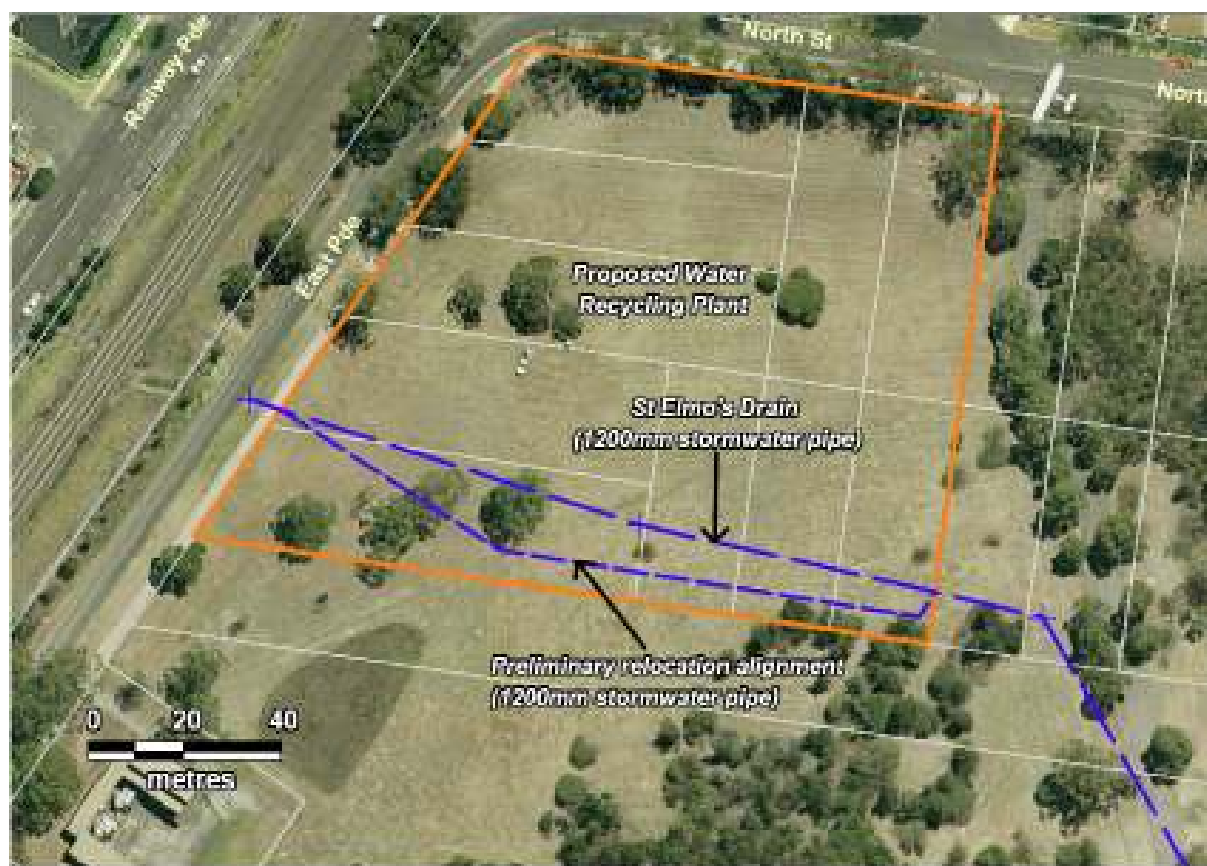
Figure 7: Preliminary relocation alignment for St Elmo's Drain
