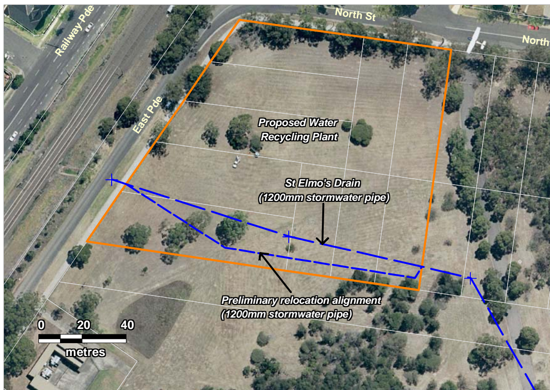
Figure 5-2 Preliminary relocation alignment for St Elmo's Drain
