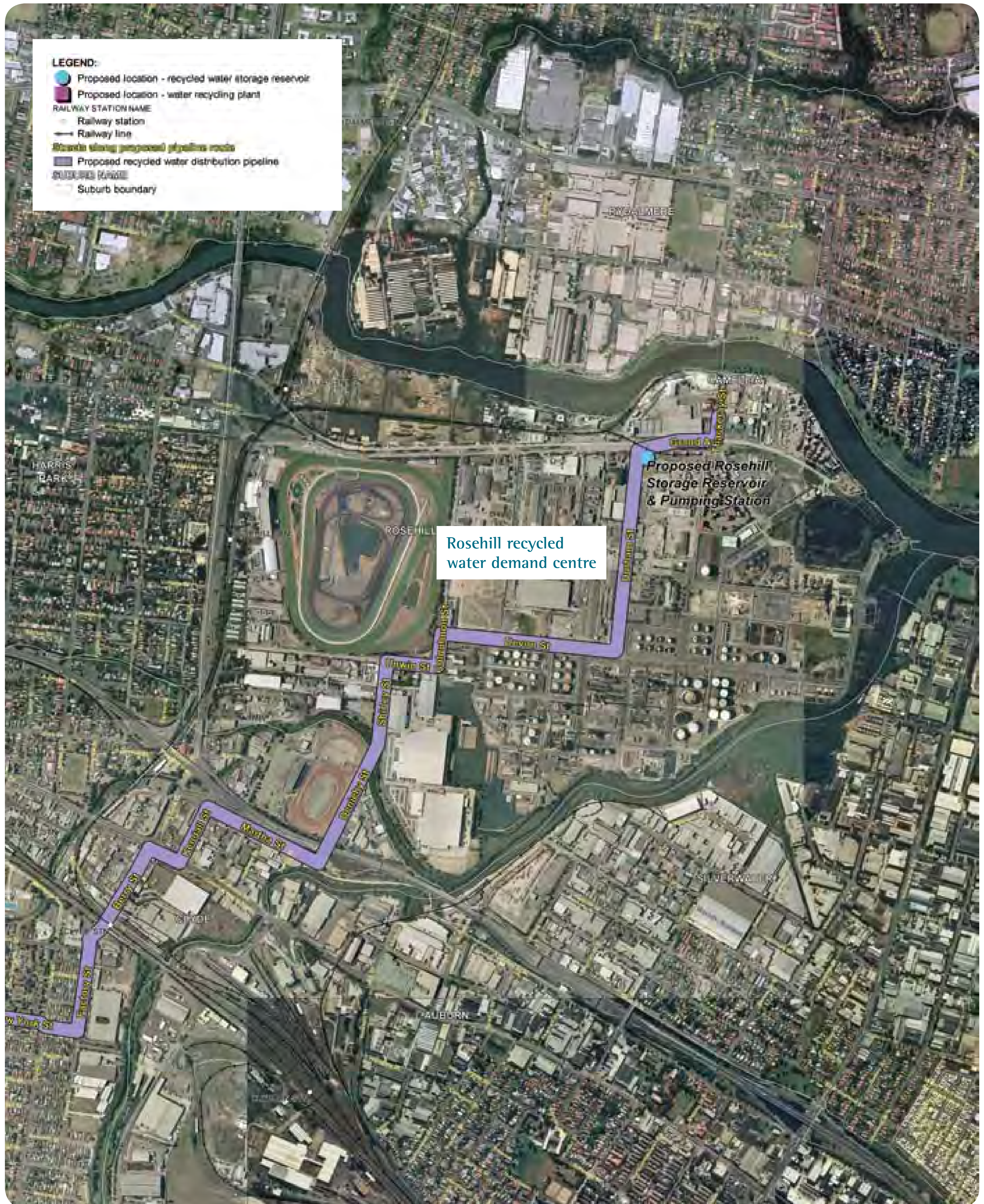
A detailed map showing the proposed route of the recycled water distribution network from Clyde to Camellia
