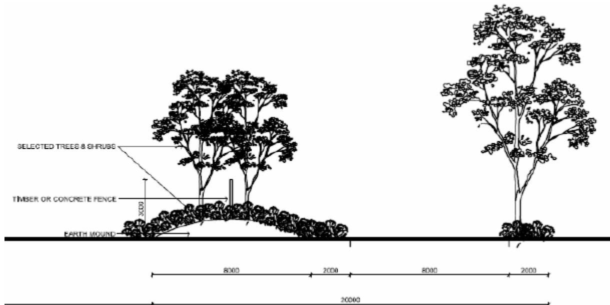
Figure 3: Detailed design of the approved acoustic bund
