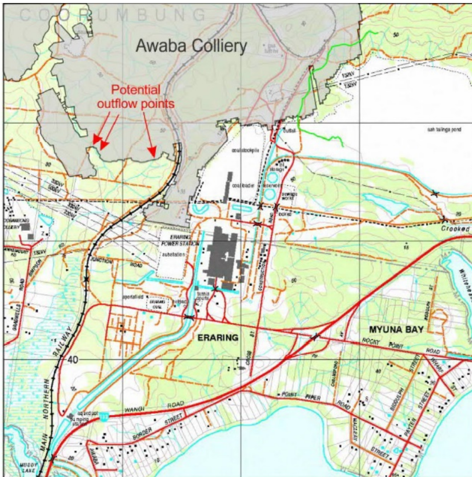
Figure 2.4 Potential water outflow points from Awaba colliery (Figure 4 from SCT, 2018)
