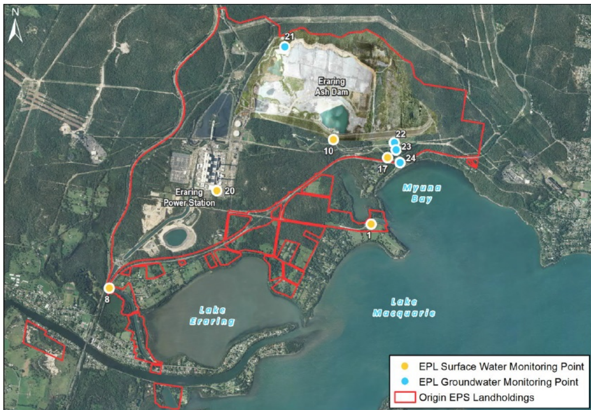
Figure 2.2 Groundwater monitoring locations (Figure 5 from AECOM, 2018a)
