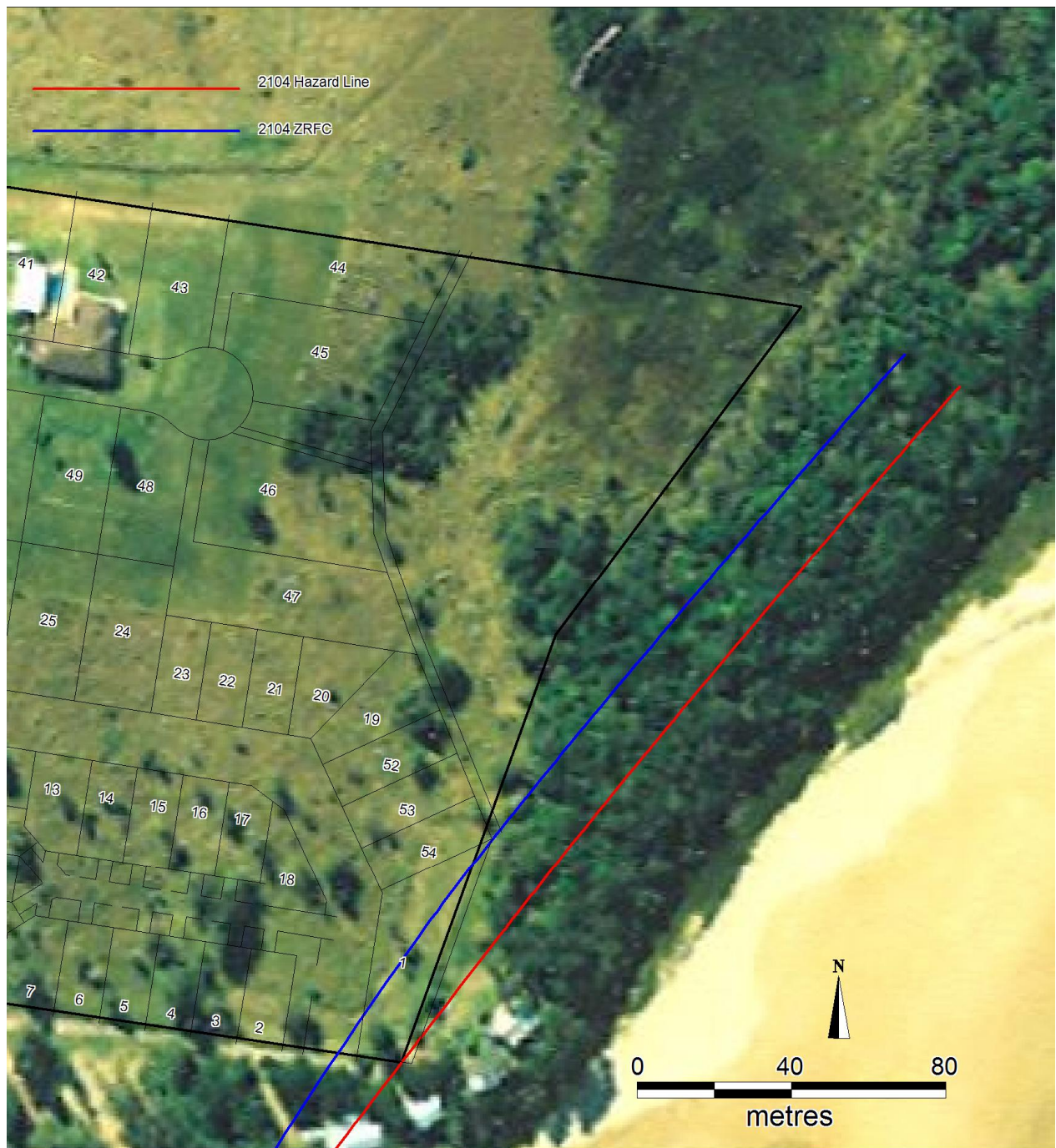
Figure 33: 2104 Hazard Line and Zone of Reduced Foundation Capacity (ZRFC) for subject property
