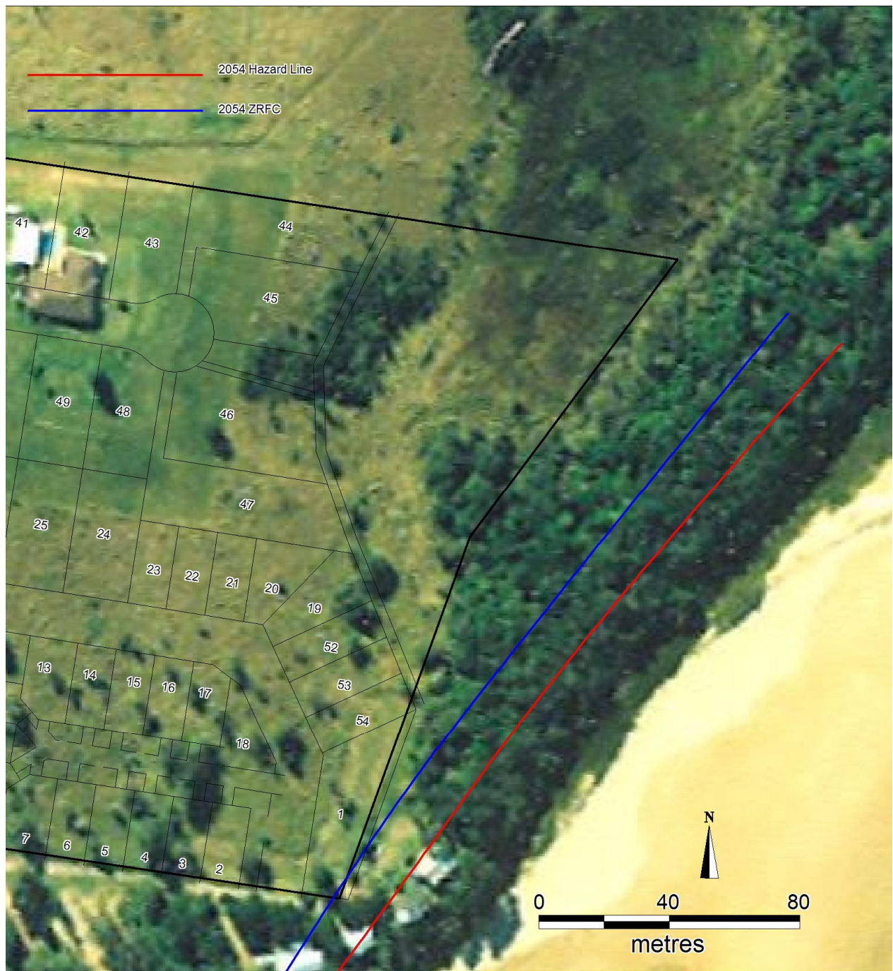
Figure 32: 2054 Hazard Line and Zone of Reduced Foundation Capacity (ZRFC) for subject property
