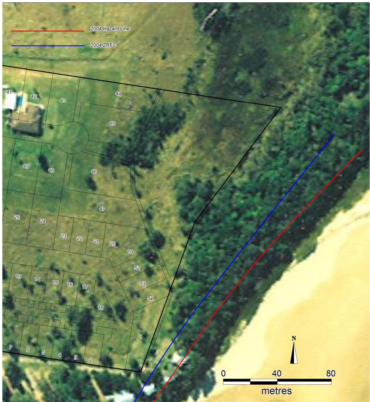
Figure 31: 2004 Hazard Line and Zone of Reduced Foundation Capacity (ZRFC) for subject property
