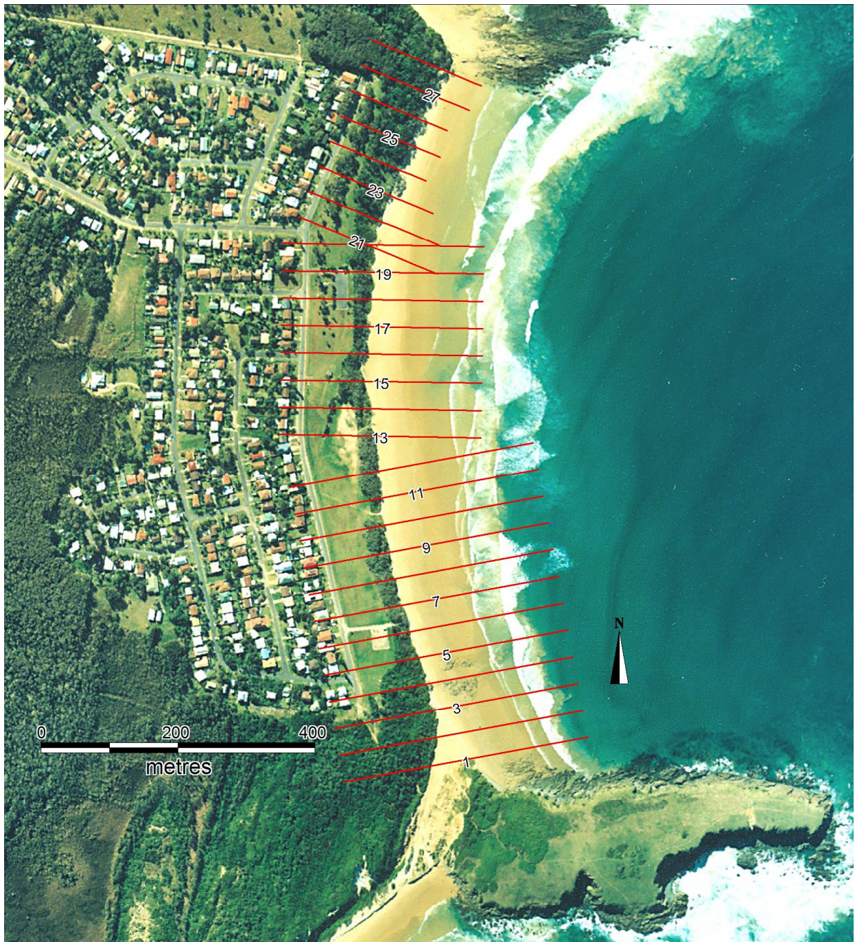
Figure 9: Arrangement of photogrammetric profiles at Sandy Beach
