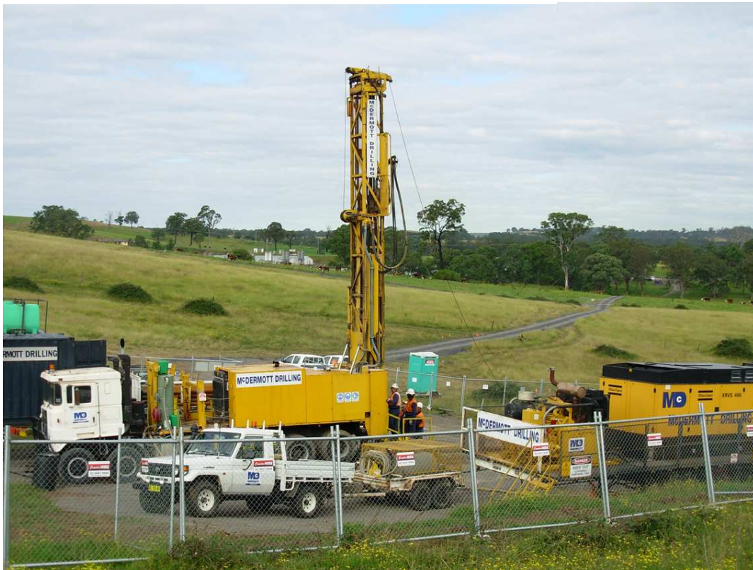
Figure 4: Photograph of trailer mounter Gas Drainage Plant
