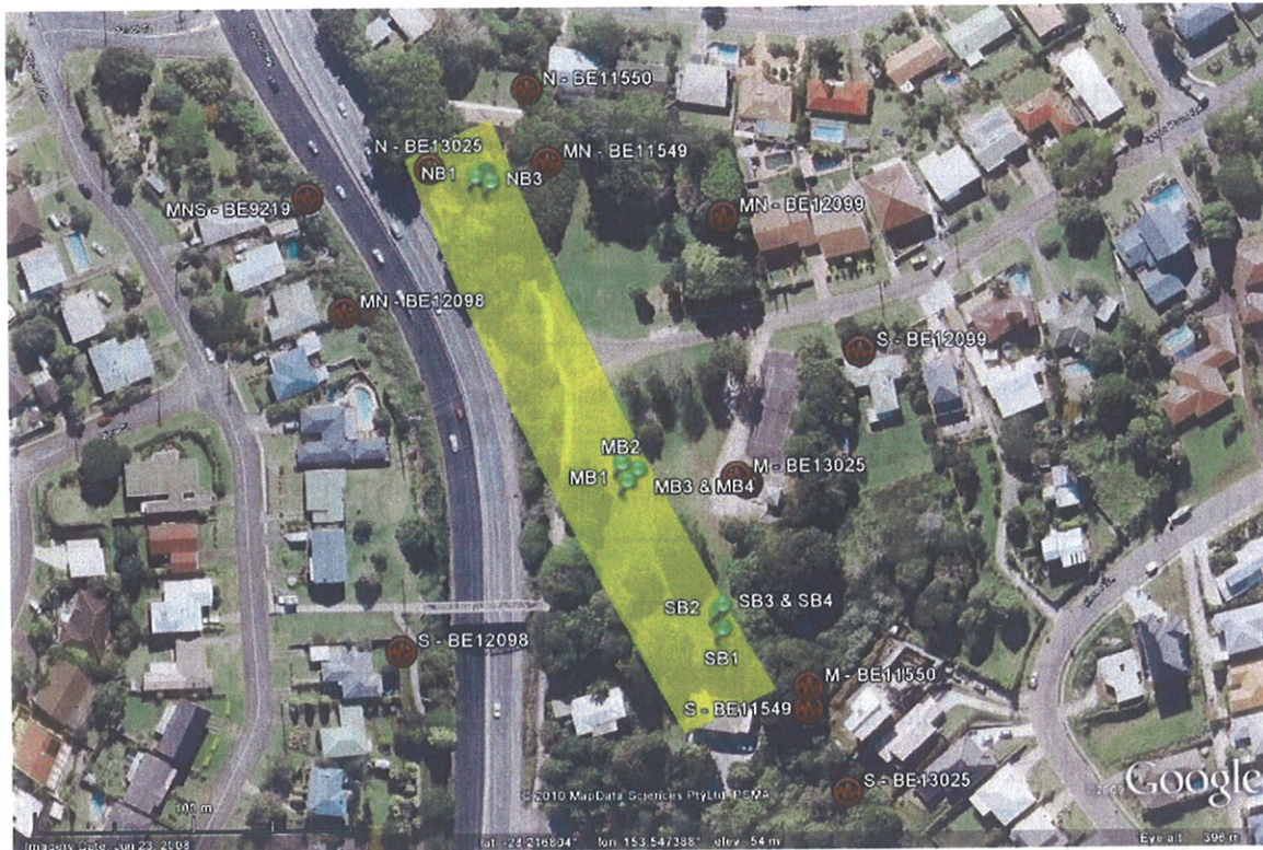
Figure 2 – Summary of monitoring and blasting locations the three trial areas. Blast locations are shown as green dots and monitoring locations as red circles with a vibration pulse
