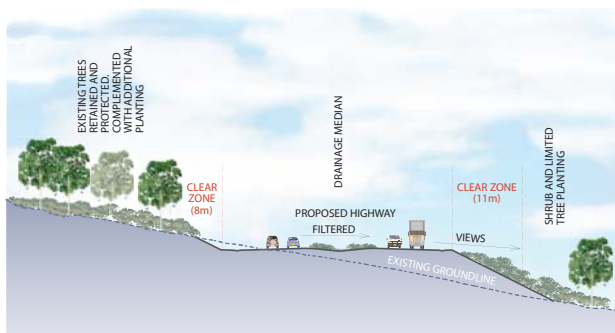
Illustration 76: Cross section at chainage 143,700
