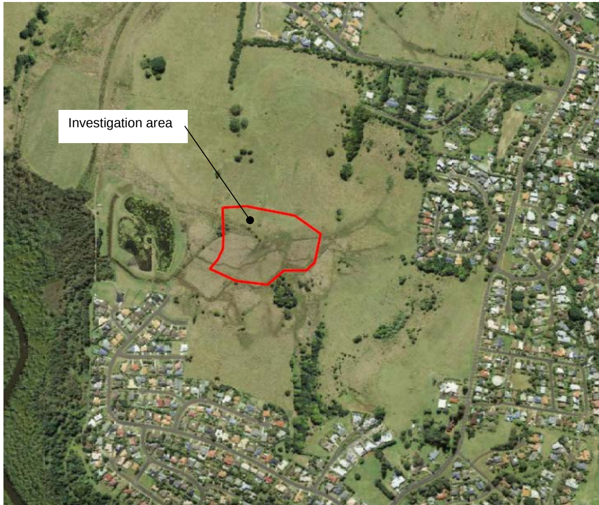
Figure 7: Aerial photo showing drainage lines prior to filling (SIX Viewer 2018)
