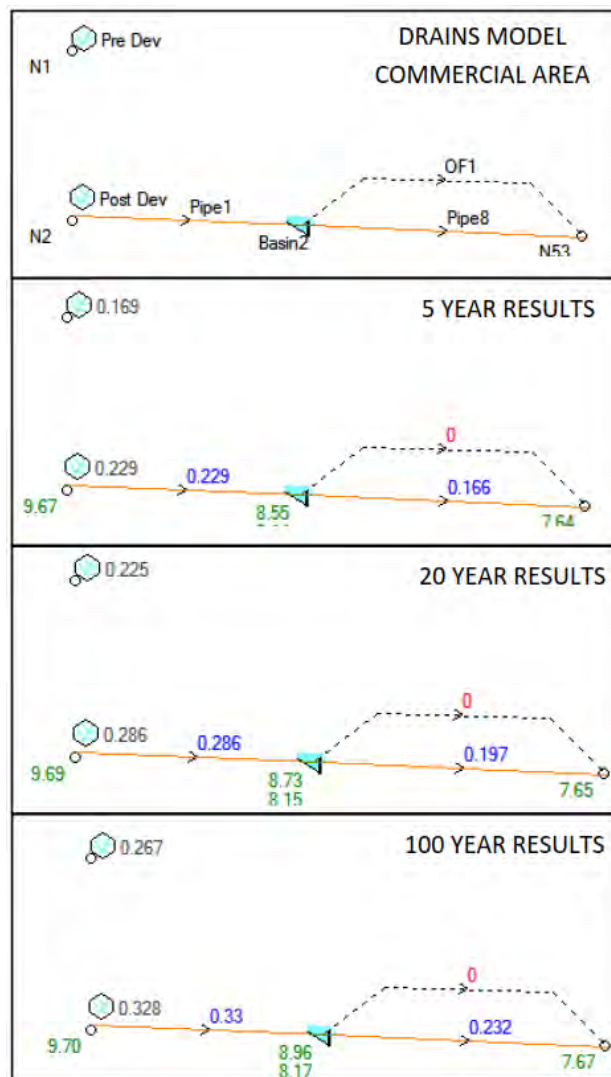
Figure 7-9 - Commercial Zone Drains Results
